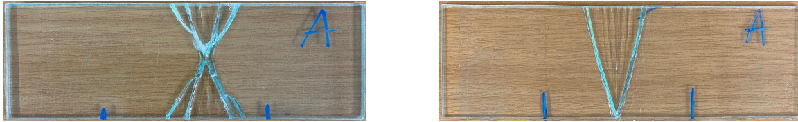
a. fracture initiation on the face
