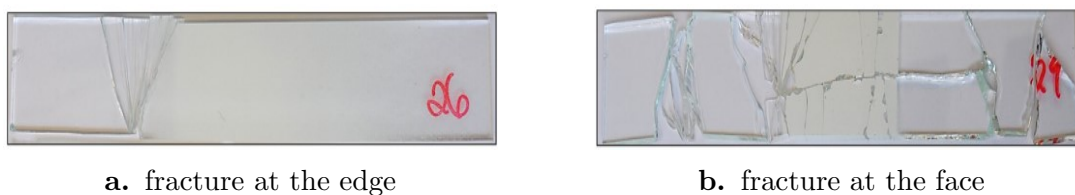
Figure 2.22 Photographs of typical glass fracture in FPBT [7]
