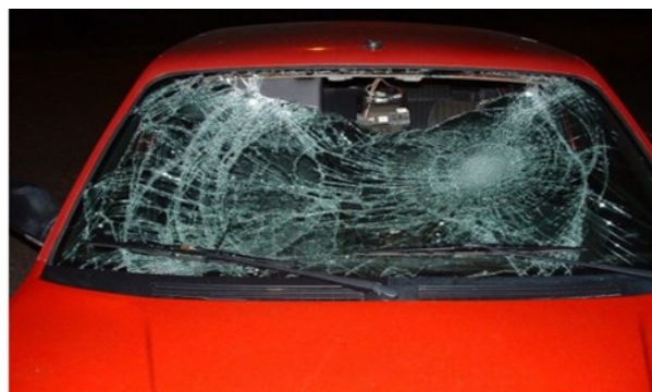
Figure 1.3 Broken windscreen of a car [13]
