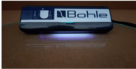
a. tin-side showing reflected light
