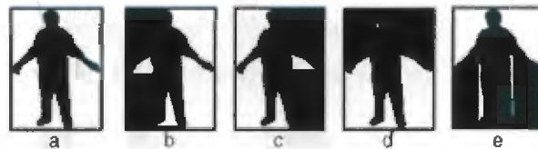
Figure 4.4: Individual images that result from the horizontal (b,c) and vertical scanning (d,e) processes.
