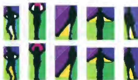
Figure 4.8: The white regions are filled with the colours of the area bordering its sides, this increases the space occupied by the colours and reserves white only for those areas completely bordered by black.
