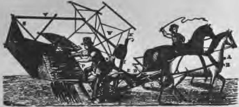
77. McCormick's Reaper. 1846. This 1850 order form shows the first model of the 'Virginia Reaper,' as it was still called, of which a series of a hundred was manufactured in 1846. The driver rides one of the horses, while the second man, riding backward on the machine, racks the grain to the ground in piles. (Library of the McCormick Historical Society, Chicago)
