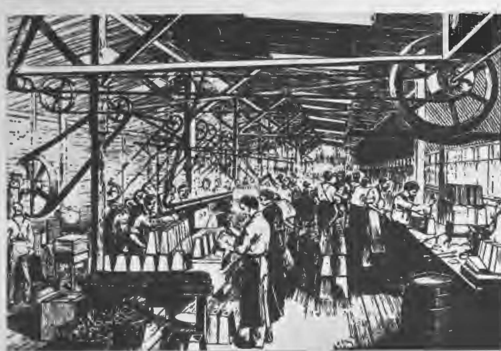
Fig. 34 Manufacture of Meat Packing Cans 1870
