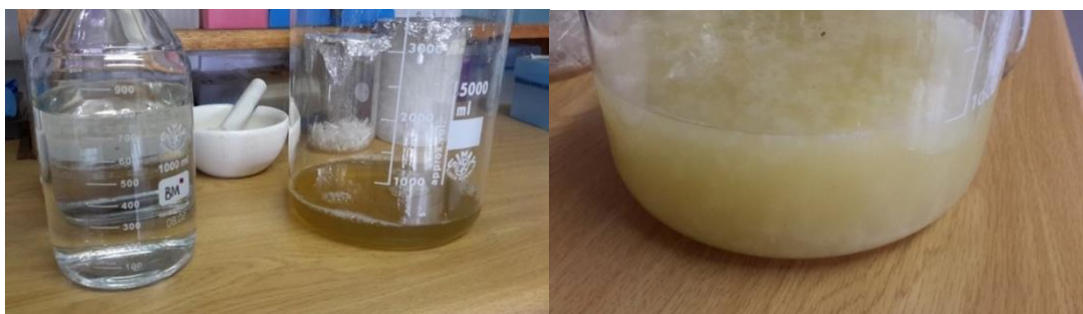
Figure 2-c The pellets were discarded and 2.5 volumes (1125 mL) of 70 % ethanol were added which precipitated out the Ulvan. After 1h the doe-like precipitate was removed and washed with 96.9 % ethanol before being centrifuged for five minutes at 5000 rpm.
