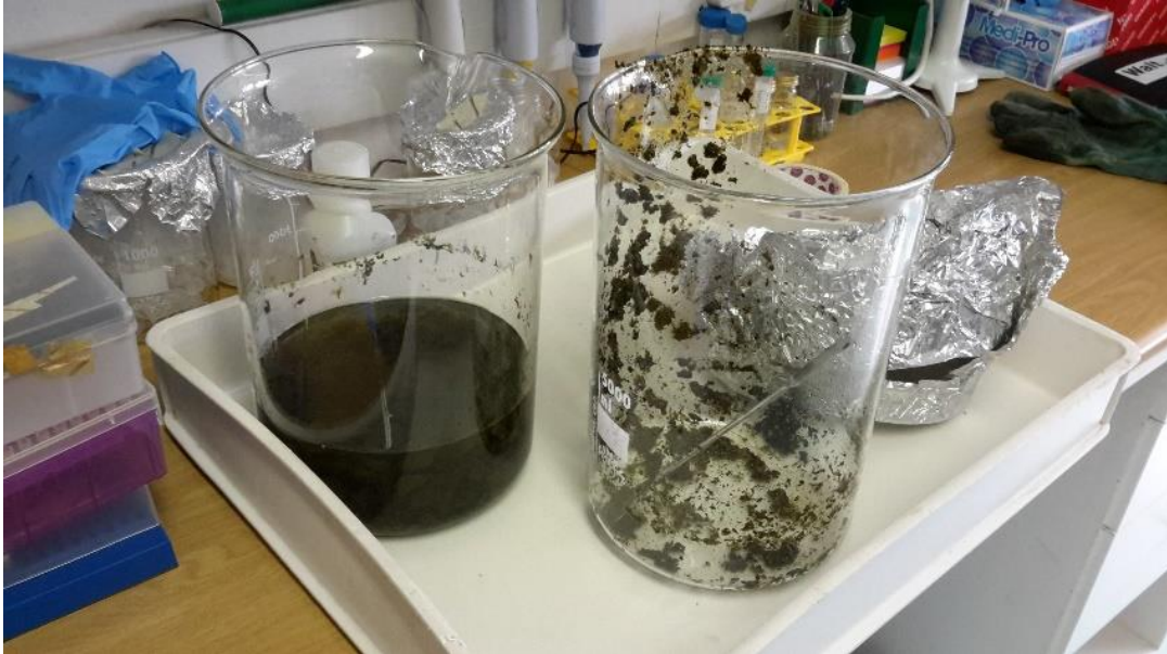
Figure 2-a Dried Ulva (50 g) was ground to pieces of approximately 1 cm. The coarse powder was then added to 450 mL diH 2 O in a 5000 mL glass beaker which was then placed in the autoclave at 120 °C for 15min.
