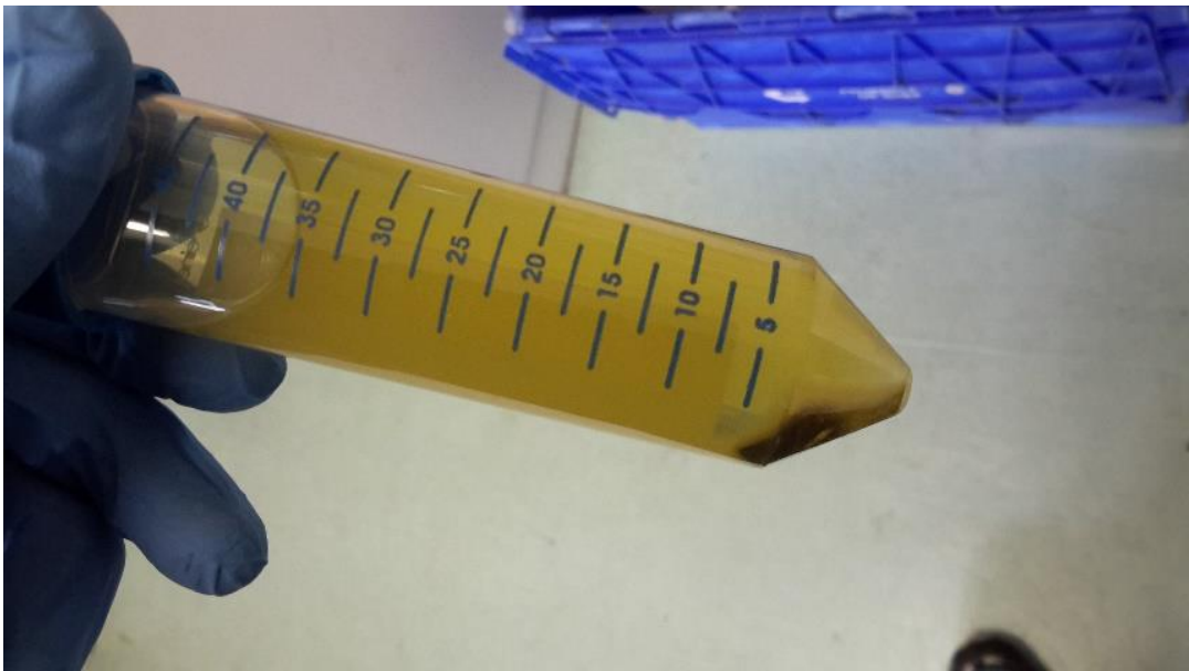
Figure 2-b The suspension was filtered through a strainer (0.25 mm) and the remaining liquid was centrifuged at 5000 RCF for 5 minutes.
