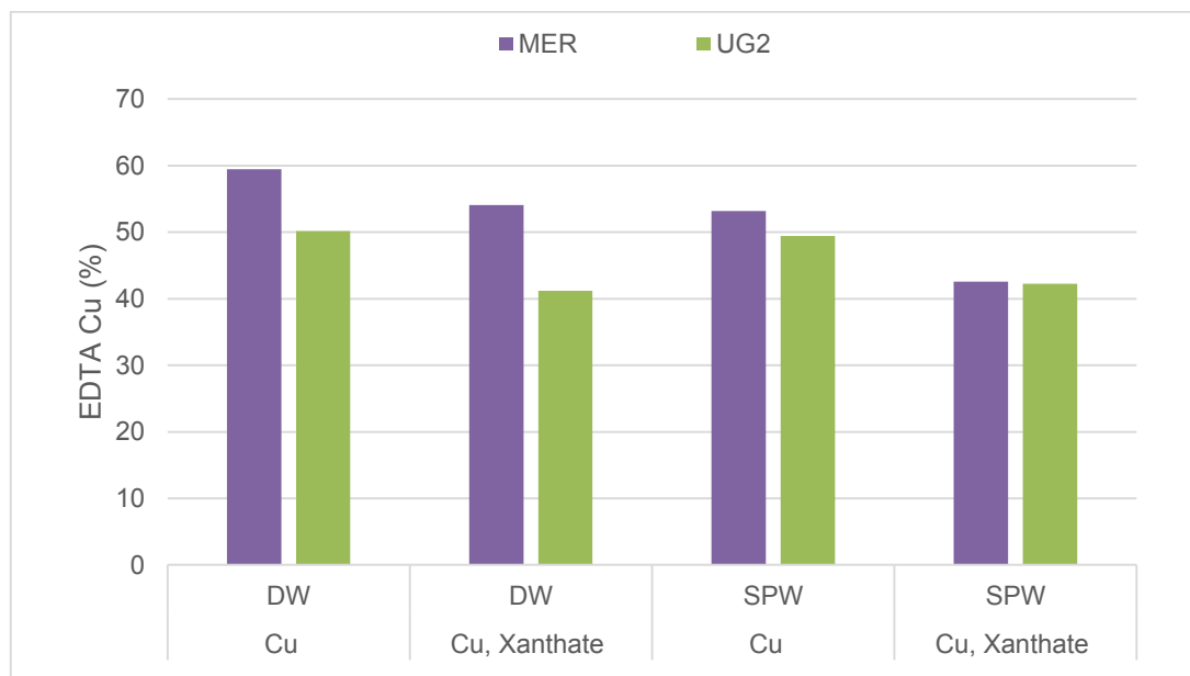
Figure 4.29: Comparison of EDTA extractable copper from Merensky and UG2 ores. The concentration of the EDTA solution was 0.03 M.
