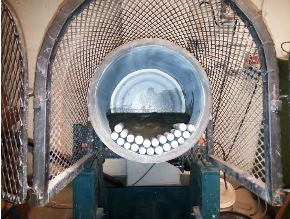
Figure 3.1: 3kg Sala rod mill loaded with wet ore.
