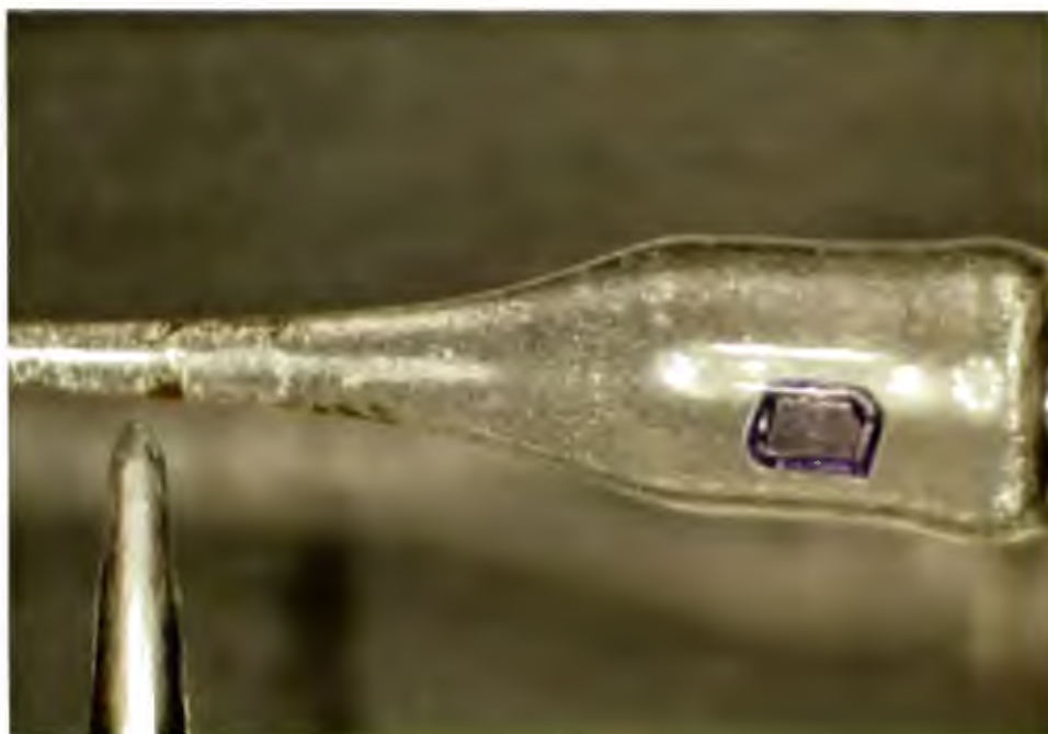
Photograph 4 The wandering crystal!! - this crystal of Compound (VIII) moved from the place indicated by the probe upwards a distance of 7mm in 24 hours.
