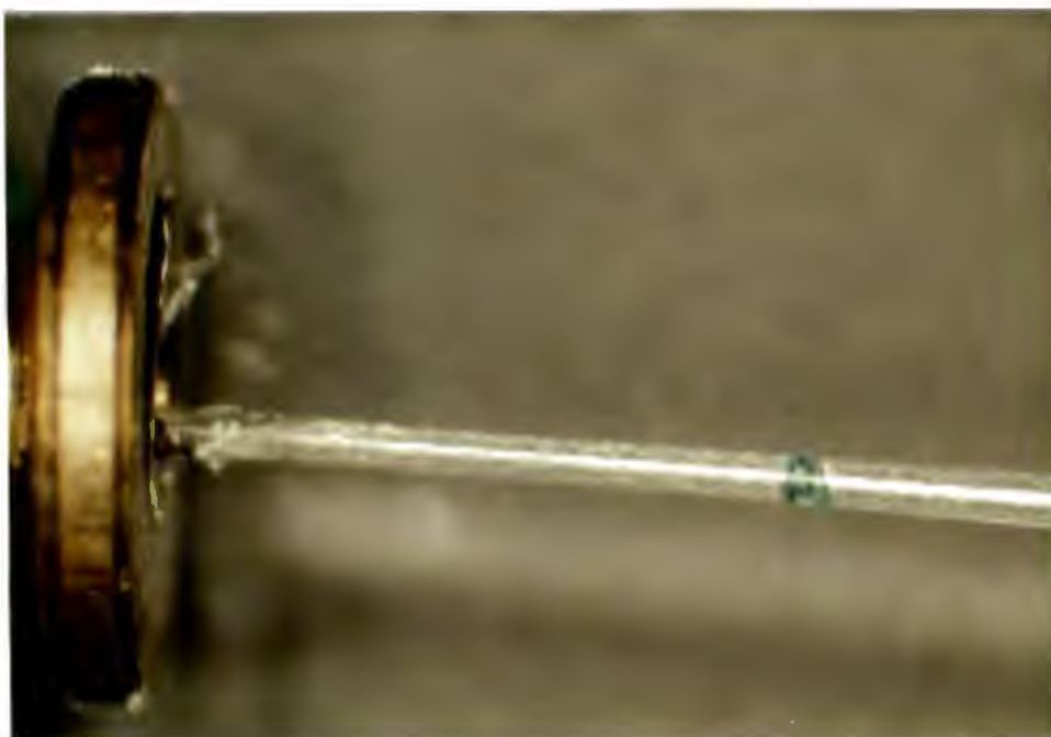
Photograph 3 A typical crystal of a clathrate mounted in a Lindemann capillary to prevent desorption of the guest.
