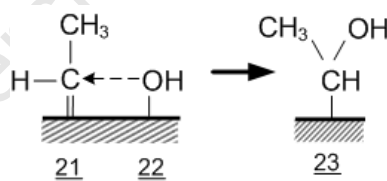
Figure 1.2 Pathway of formation of surface oxygenates from Johnston and Joyner (1993)
