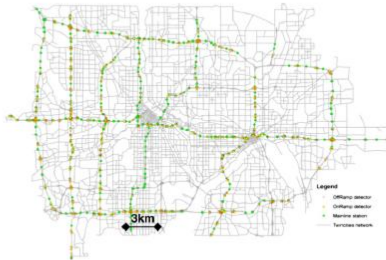
Figure 2.10: Chosen location in Minnesota for the study, with the green dots representing the loop detector locations.
