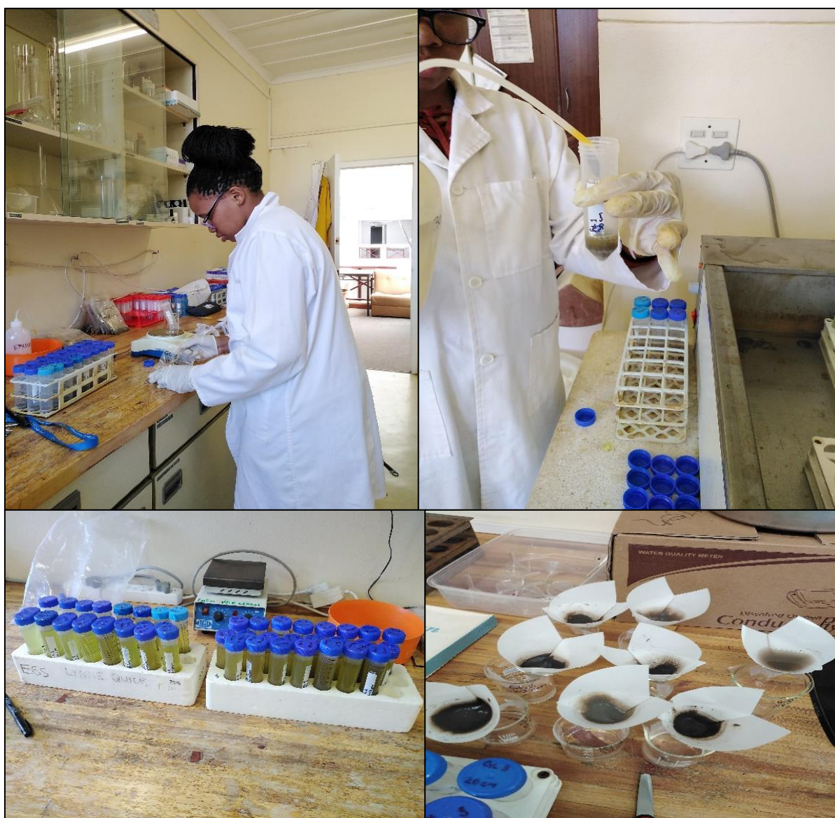
Figure 4.6: Process of removing carbonates in the soil samples using HCl. Pictures taken in October 2019.
