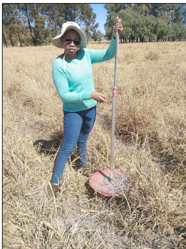
Figure 4.5: Measuring grassland biomass using disk pasture meter. Picture taken in September 2019
