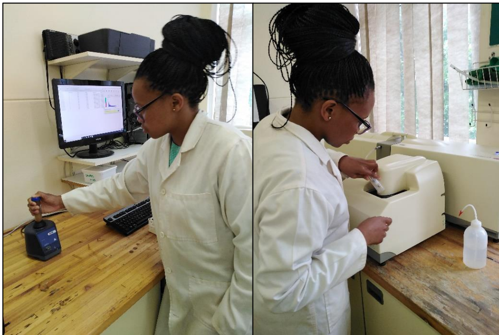
Figure 4.7: Measuring the grain sizes distribution using Malvern Mastersizer 2000. Both pictures showing the process of measuring grain size. Pictures taken in November 2019.
