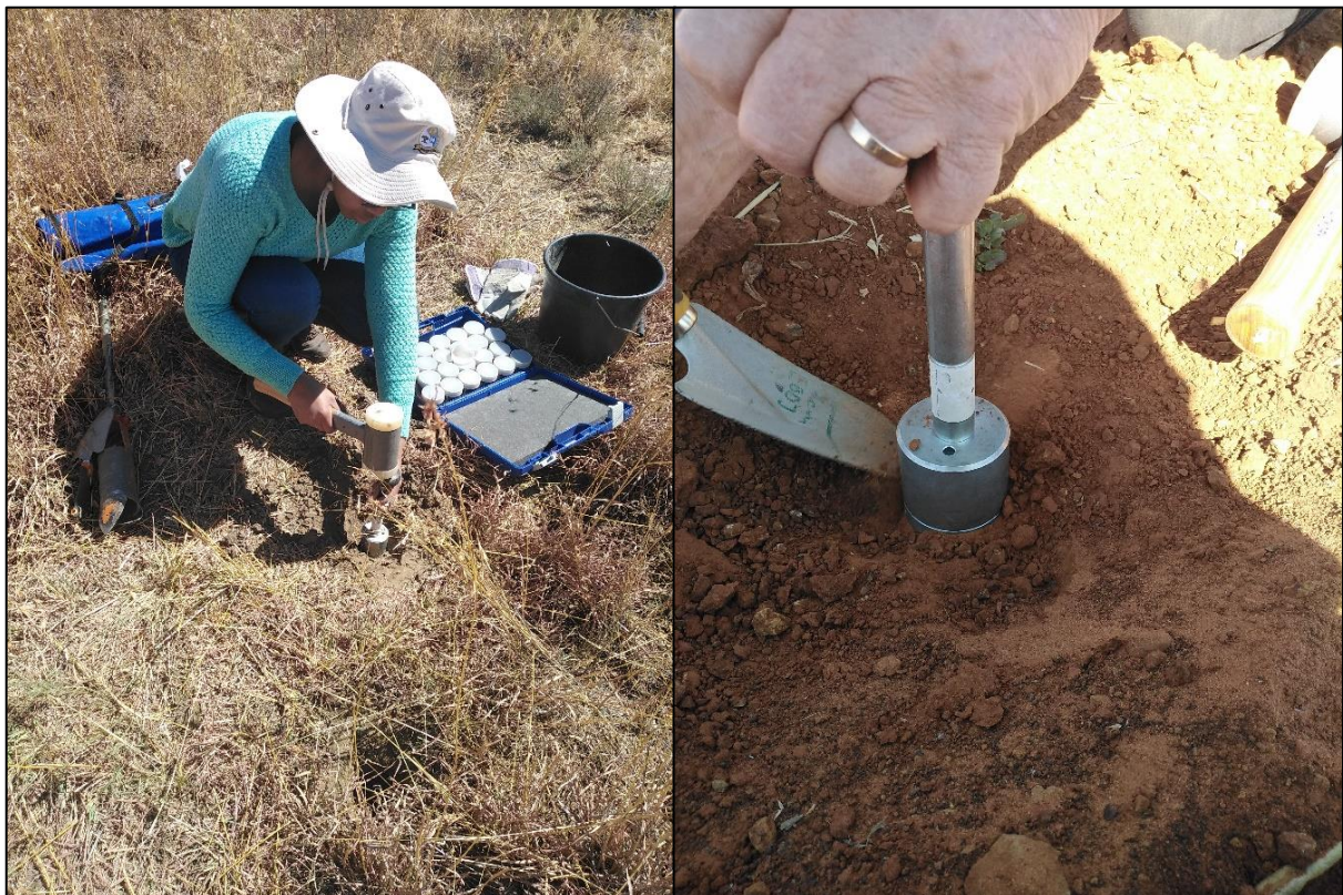
Figure 4.4: Measuring bulk density. Both pictures showing the procedure to get the bulk density soil sample. Picture taken in September 2019
