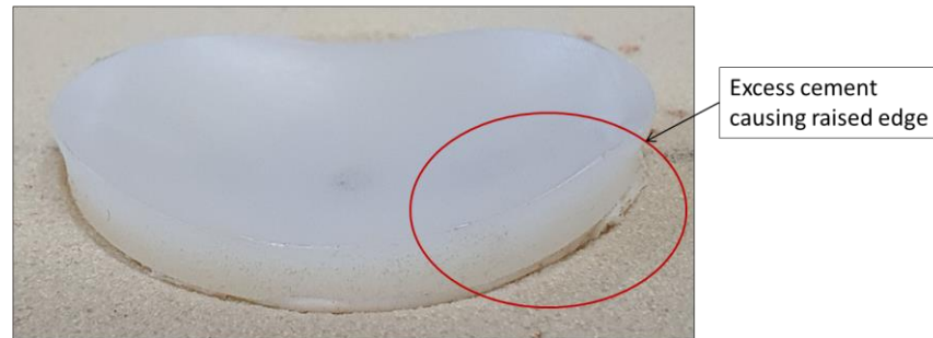
Figure 2-31 Expired size 52mm glenoid sample used in the P90 test validation, which has unevenly distributed cement, causing the subluxation distance to not be symmetrical around the glenoid centroid.
