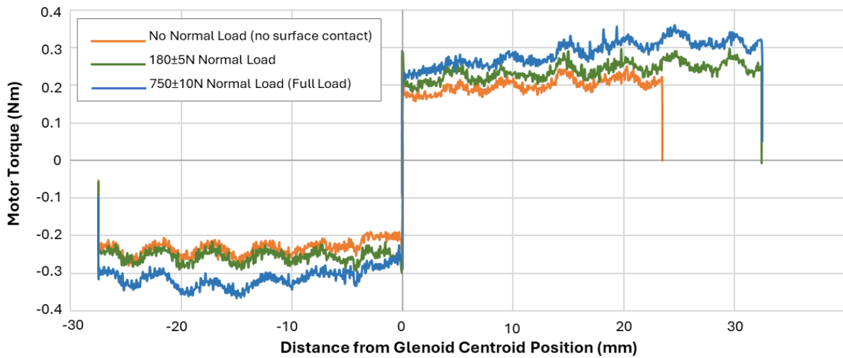
Figure 2-23 Measured motor torque for motion at a constant speed (50mm/min) on a flat surface, for three load conditions, in both directions away from the position the glenoid centroid would be mounted.
