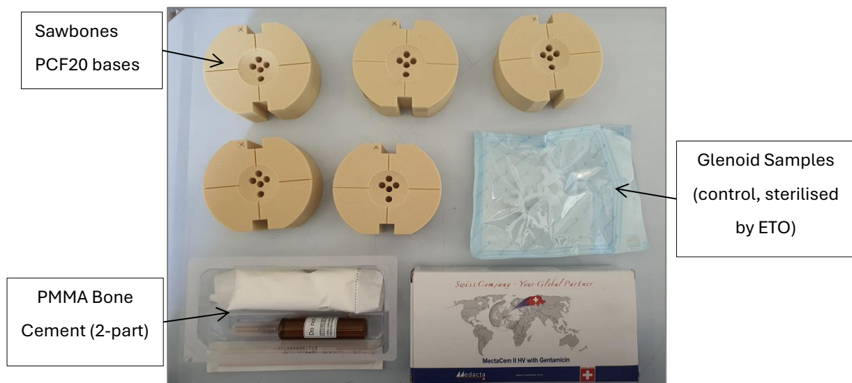
Figure 4-5 Materials used in the implantation of the glenoid samples (control glenoid components shown)
