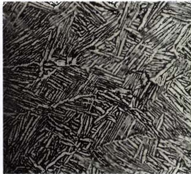
Figure 2.3b: Ti-6Al-4V, forged at 1038°C above the beta transus, air cooled, annealed for 2 hr at 704 °C, and air cooled showing a Widmanstätten structure 31 .
