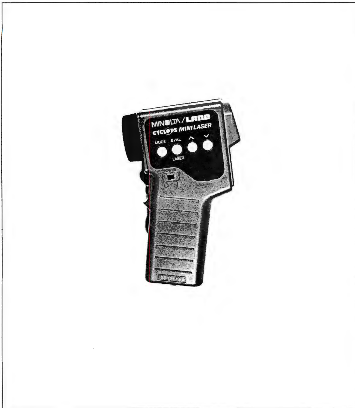
Figure 3.34 The infra-red mini-laser temperature sensor
