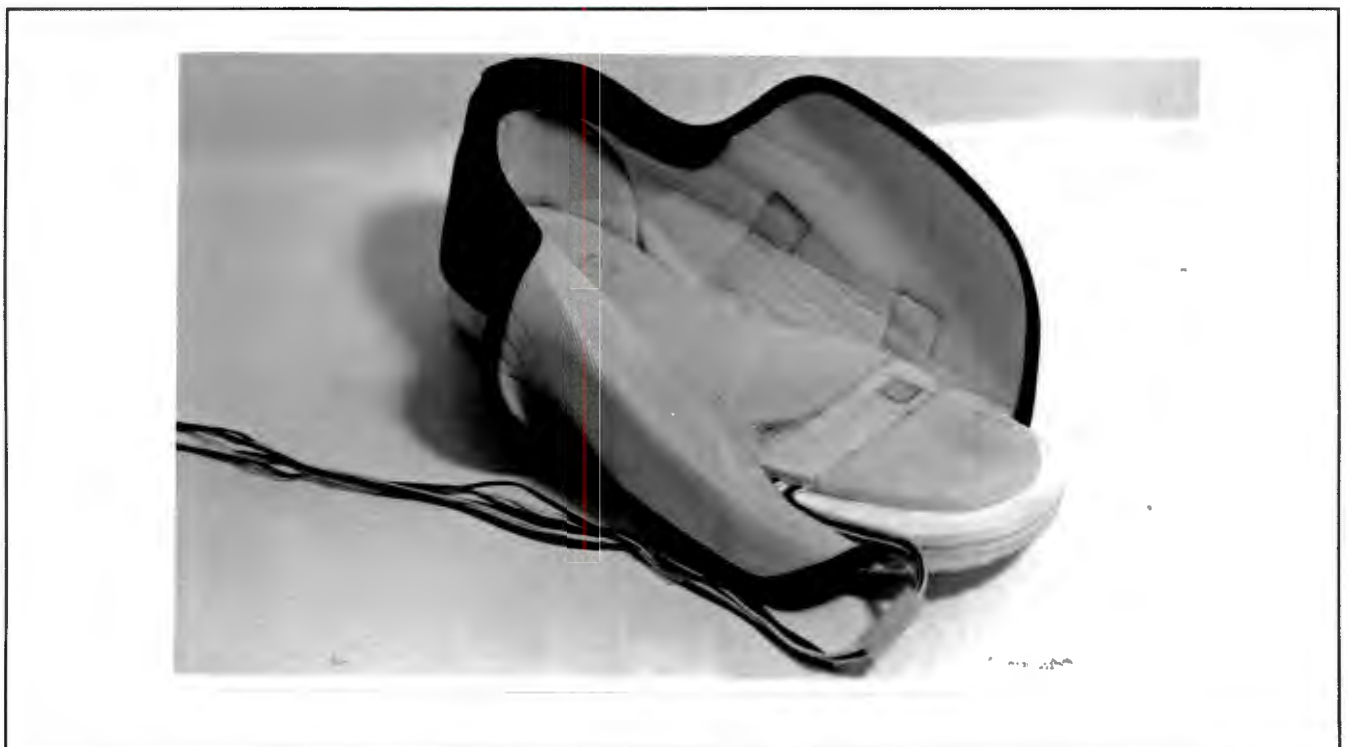
Figure 3.31 Illustration of the new instrumented insole fitted to the standard (See text, page 115) diabetic shoe
