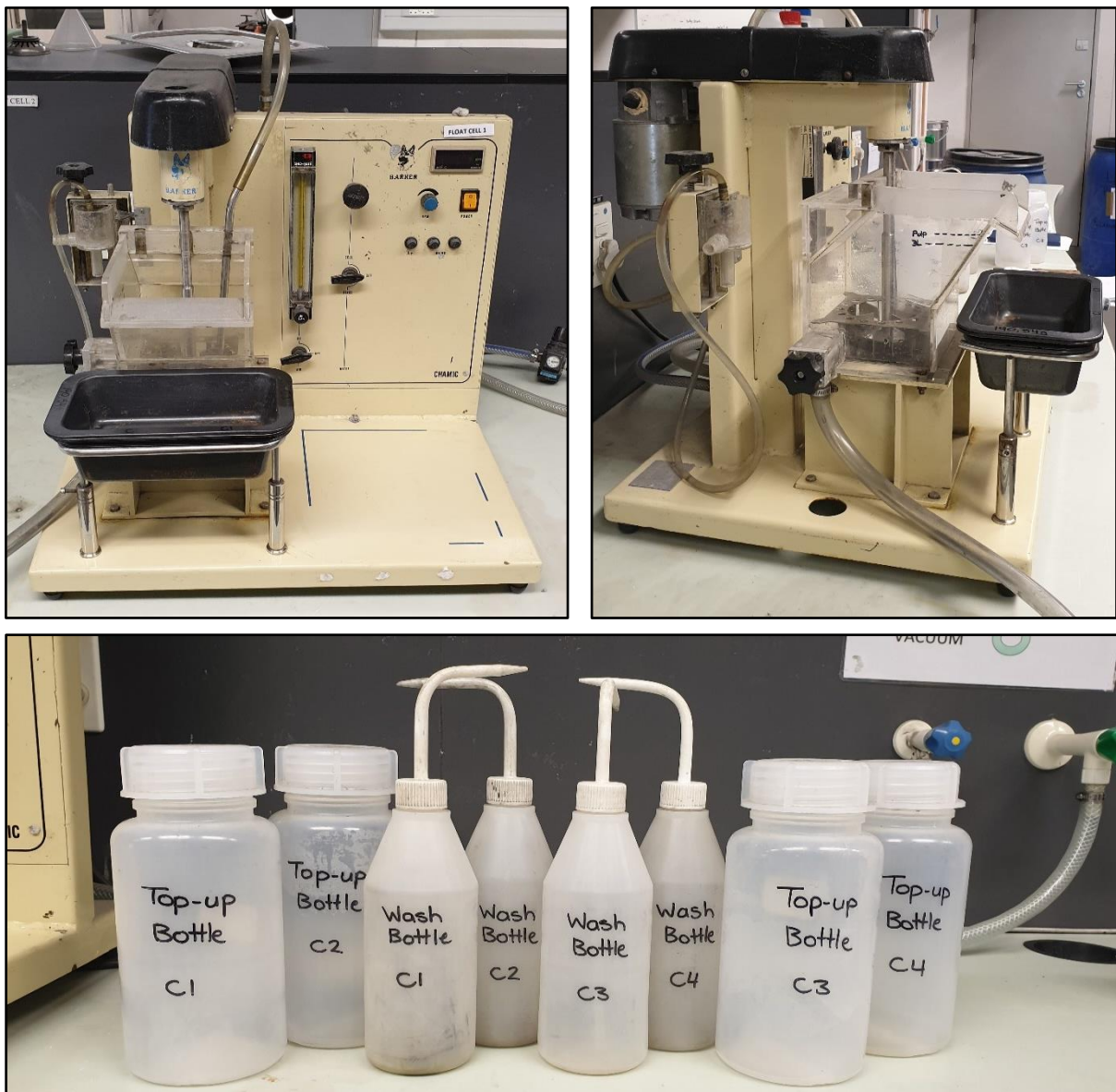
Figure 21 - Images of the 3L modified Leeds flotation cell and accompanying bottles
