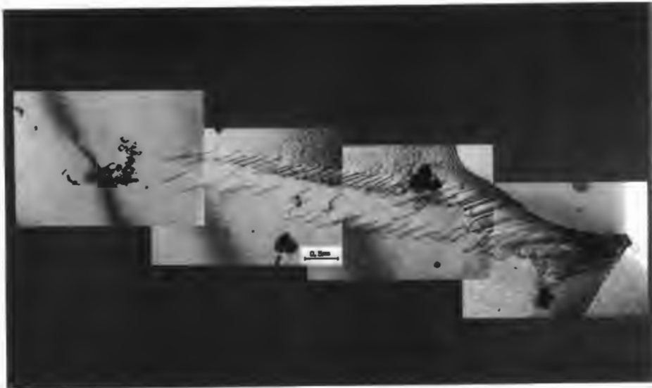
Figure 56: Bright-field TEM micrograph collage illustrating the emission of a planar dislocation array from a triple point junction. The foil was machined from a specimen where deformation was interrupted prior to macroscopic yielding in the gauge length.
