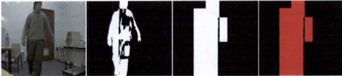
Figure 24: The use of filled rectangles to represent blobs
