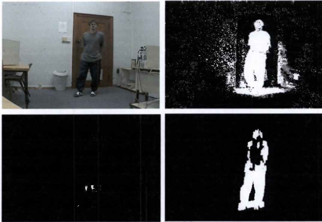
Figure 4: The effects of various threshold values
