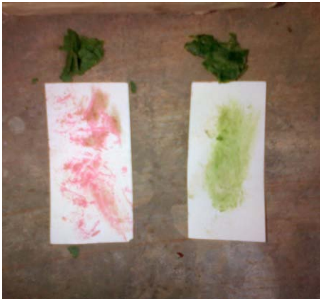
Figure 2.2: DMG-indicator paper Ni test. Presence of nickel ( \text{Ni}^{2+} ) within leaf cells was determined by smearing broken leaf tissue directly onto indicator paper (on site) from hyperaccumulator (left) and non-accumulator (right) plants, respectively. Colour development occurred instantly on contact with leaf Ni.
