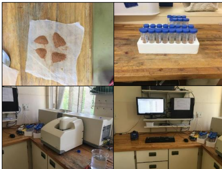
Figure 4.3: Laboratory photographs of: Top left: The sediment quartering process. Top right: The sediment samples diluted in test tubes prior to Malvern analysis. Bottom left: the Malvern Mastersizer 2000, composed of the dispersion unit in the foreground and the Malvern in the background. Bottom right: The operating computer for the Malvern with the small centrifuge on the left
