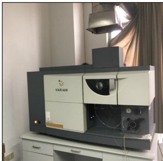
Figure 4.11: Photograph of the Agilent Varian 710 ES ICP-OES machine used for heavy metal quantification
