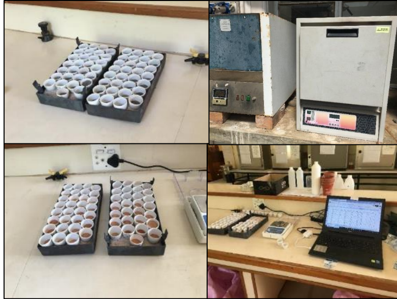
Figure 4.2: Top left: Photograph of the crucibles in their furnace trays, prior to entering the furnace. Top right: Photograph of the two muffle furnaces used for LOI. Bottom left: Crucibles with TOC removed after the LOI process. Note the colour change from the top left image. Bottom right: The system used to weigh and record the mass of the sediment samples
