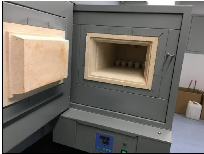
Figure 4.7: Photograph showing the interior of the muffle furnace used for loss on ignition analysis
