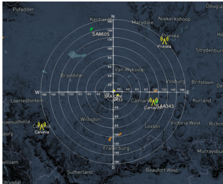
Figure 3.7: A screenshot of the MeerKAT RFI monitoring system. The MeerKAT array is denoted by the yellow dot at the centre. The yellow tower-like structures are the communication towers and the blue dot at around 350° azimuth is a flying aircraft. The annuli represent the distance from the core in km.
