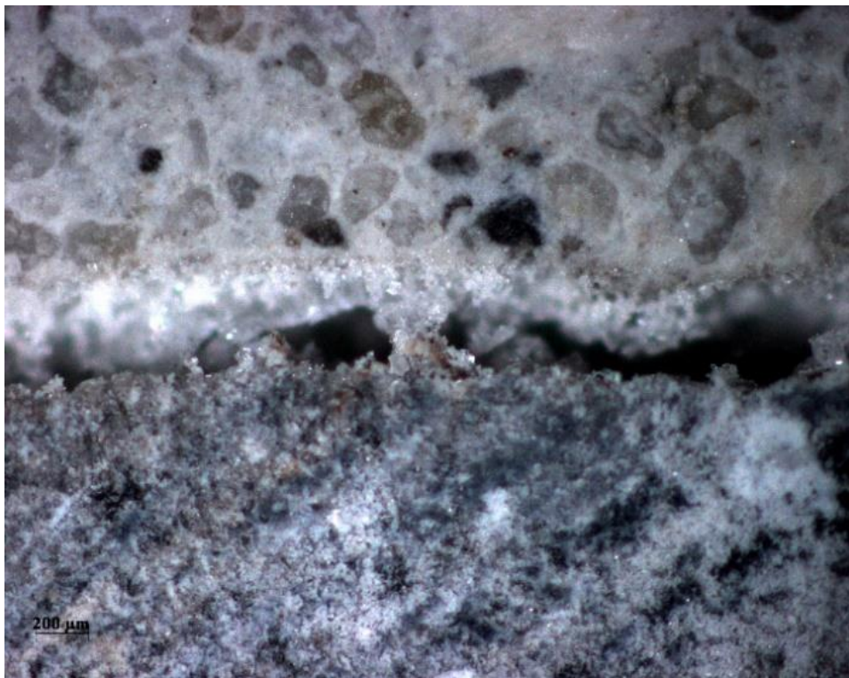
Figure 4-29: CA-3 self-healing crystals observed through an optical microscope
