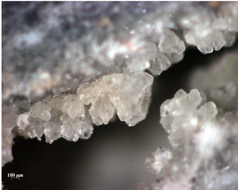
Figure 4-26: Control concrete self-healing crystals observed with an optical microscope
