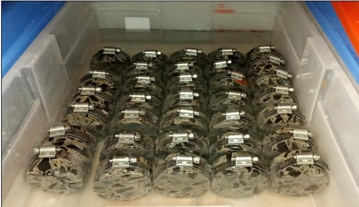
Figure 3-4: Curing of the cracked specimens
