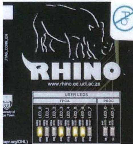
Figure 6-2: LEDs indicating a value of 300 on the pulse length register.
