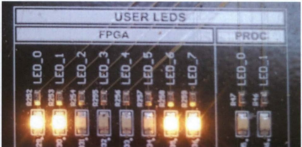
Figure 6-1: Photo of FPGA LEDs during operation of "Rhino_Blinky"
