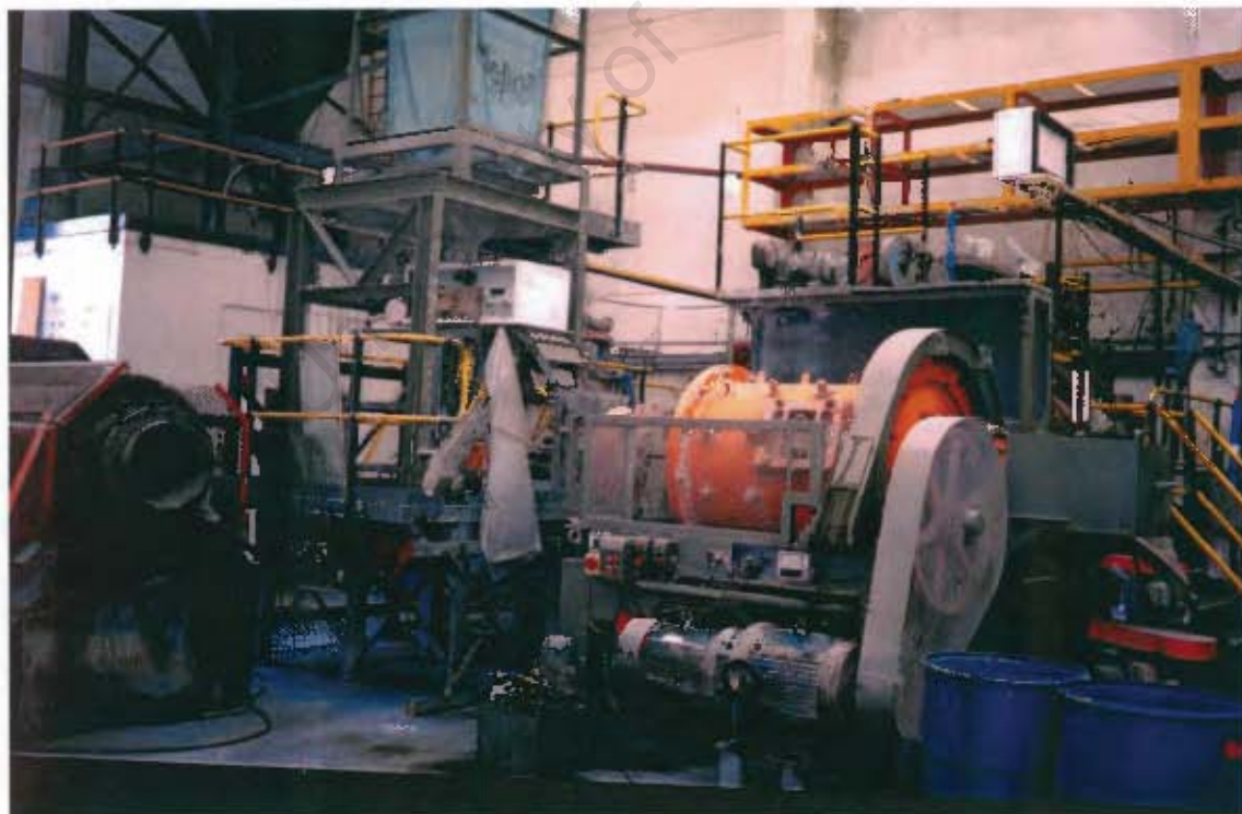
Figure 4.7: Photograph showing the mill and mill feed assembly for the test work of phase I
