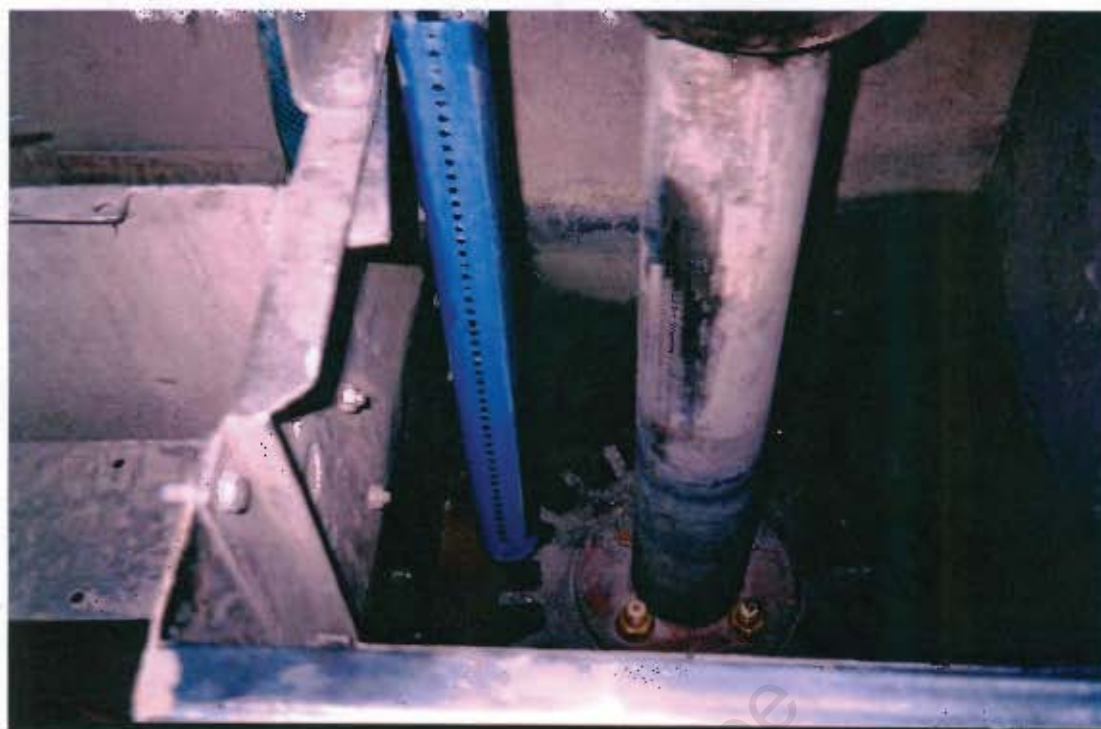
Figure 4.5: Photograph showing the position of the digilevel in a flotation cell on the pilot plant
