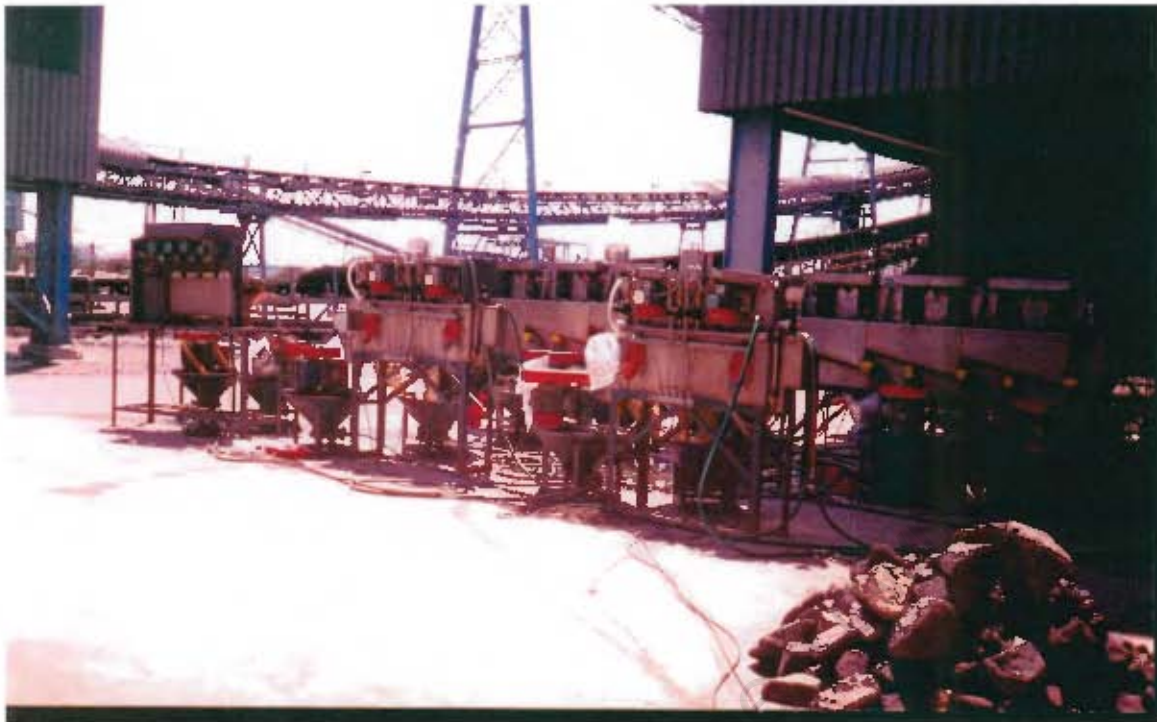
Figure 4.1: The Mintek flotation pilot plant at Eastern Platinum Mines
