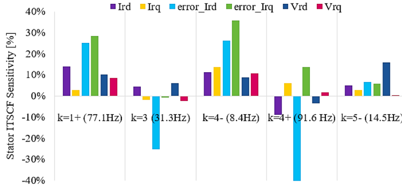
Figure 7. 8: Sensitivity study results of the Stator ITSCF-related frequency components in the DFIG controller signals, for a micromachine at medium load
