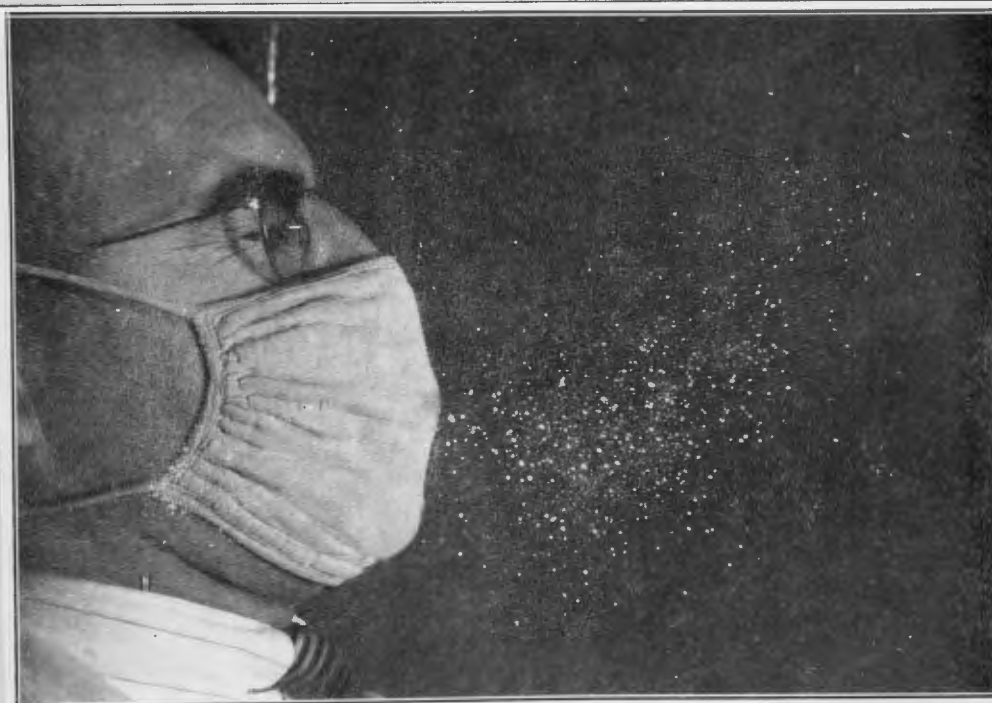
Sneezing test of an all-fabric face mask. This mask was comparatively dense, having an air-permeability less than one-fifth as high as that of the most permeable mask tested.
