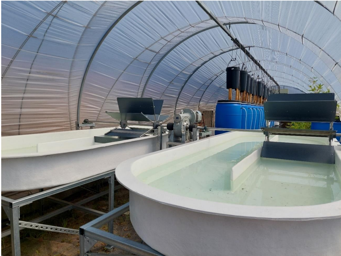
Figure 12 A picture of the 1000 L raceways used inside the University of Cape Town greenhouse. The ponds that were manufactured are identical and the paddlewheels are powered by a single motor as shown above.
