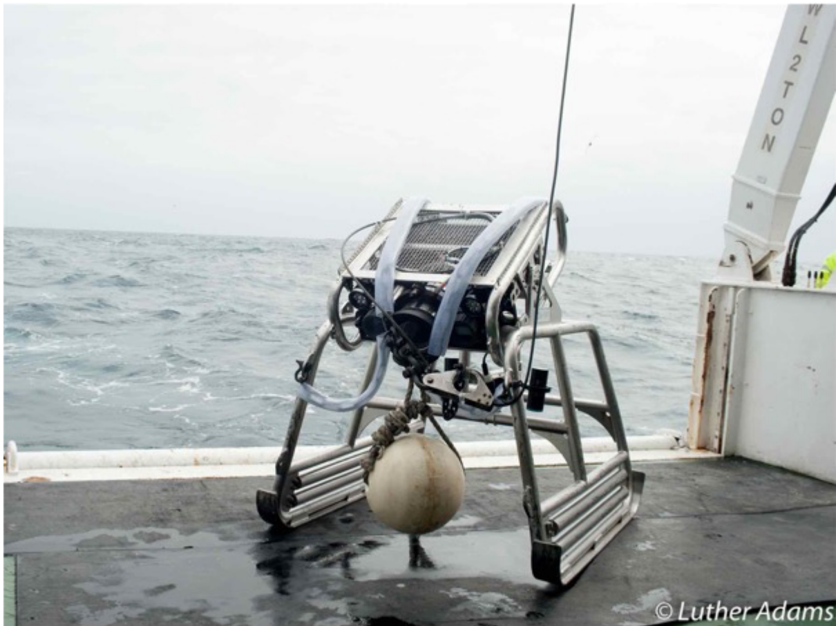
Figure 2.3 The Ski-Monkey II towed camera system. Source: L. Adams, 2018.
