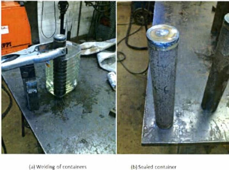
Figure 4.10: (a) Sealing of samples in steel containers and (b) sealed container
