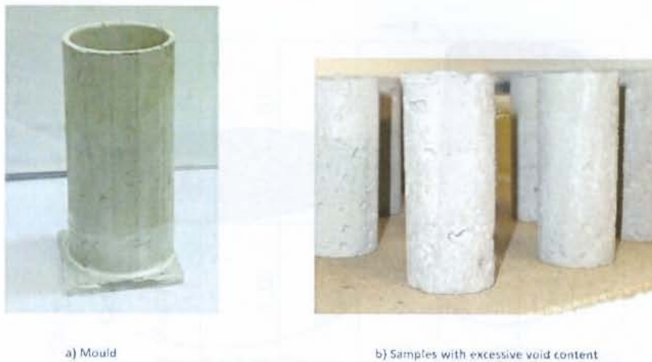
Figure 4.3: Mould attempt 1: (a) mould and (b) samples with excessive void content
