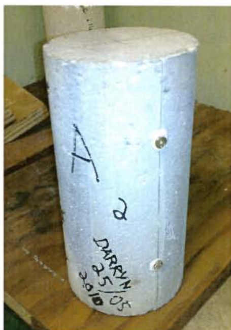
Figure 4.14: Shrinkage sample with points mounted
