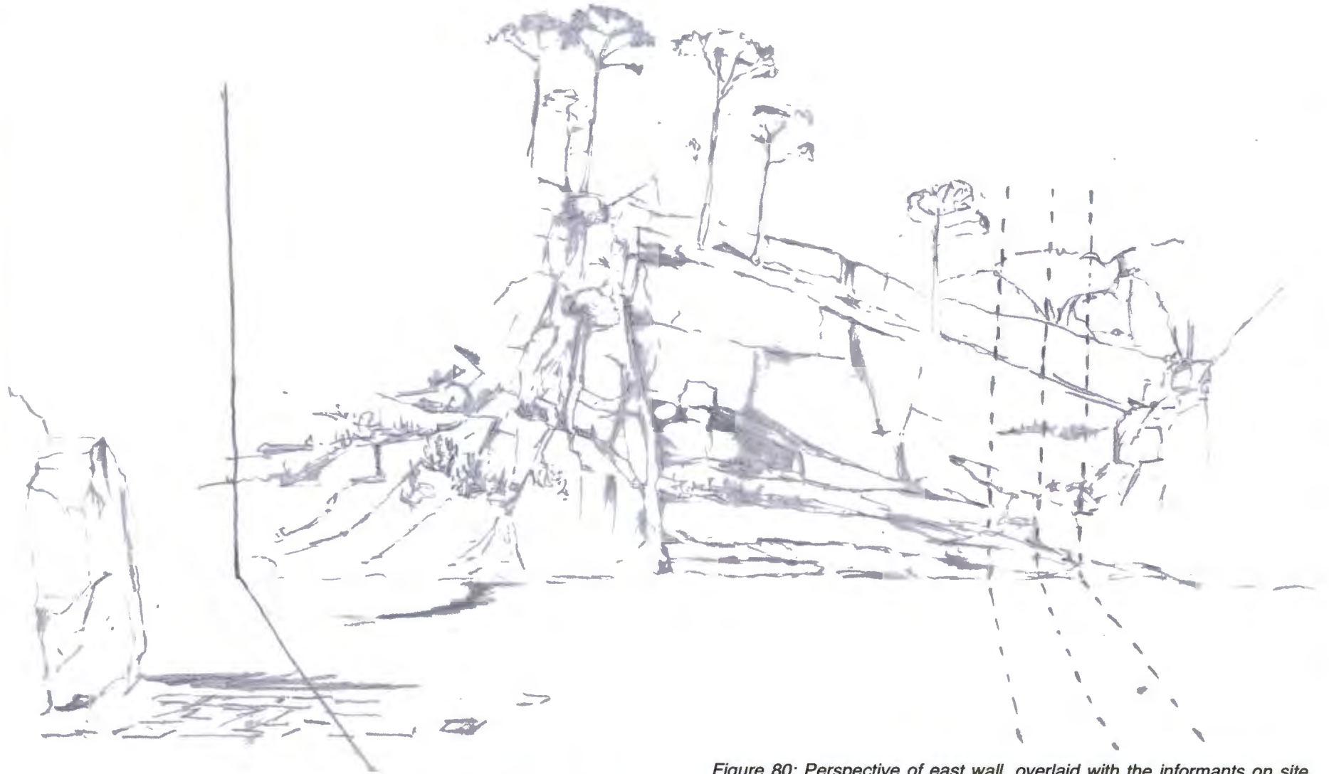
Figure 80: Perspective of east wall, overlaid with the informants on site, such as drill lines (dotted line on the right), orientation of quarry face and the remnant wall structures.
