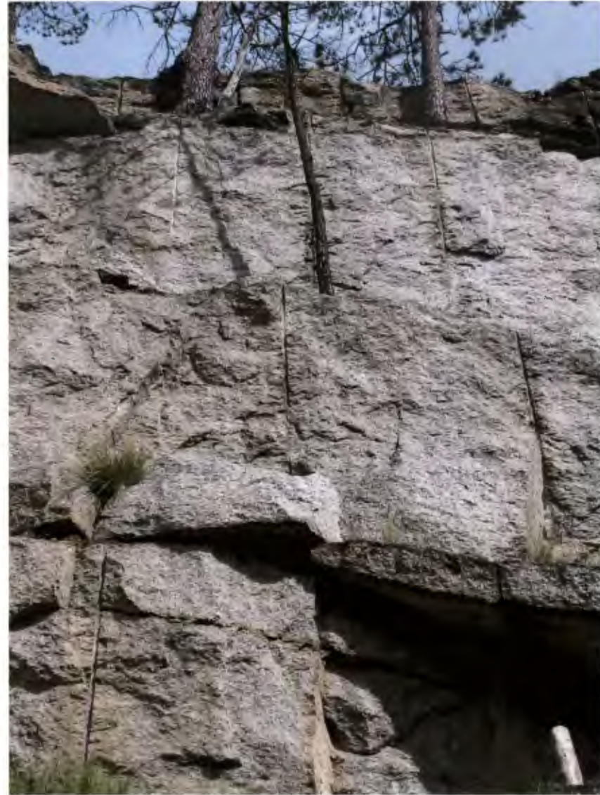
Figure 26: Drill lines in the east facing wall of the quarry, roughly 1.5 - 2 meters apart.
