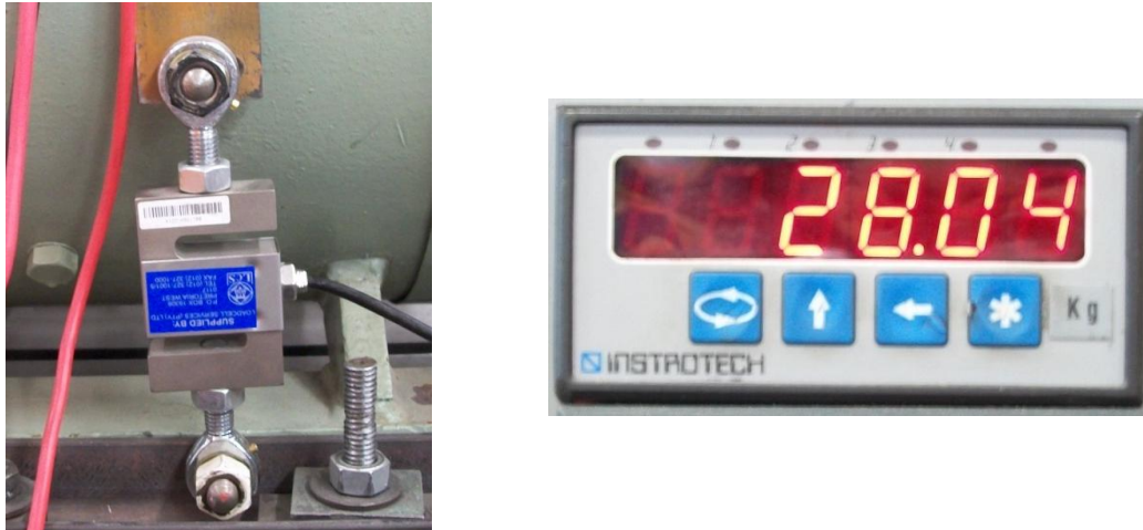
Figure 7.4: Load cell and digital torque display
