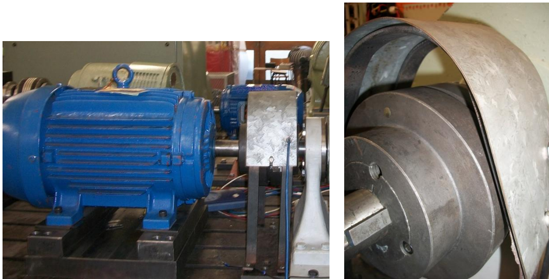
Figure 7.15: Proximity sensor placed over shaft coupling
