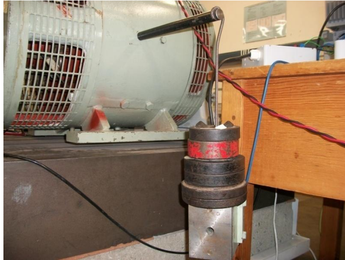
Figure 7.3: Dynamometer torque arm with weights
