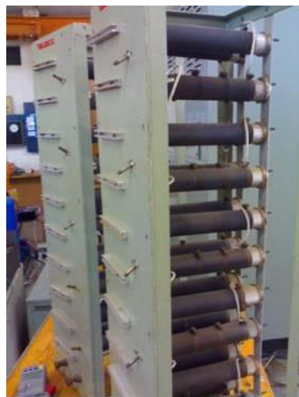
Figure 7.5: Additional load resistors
