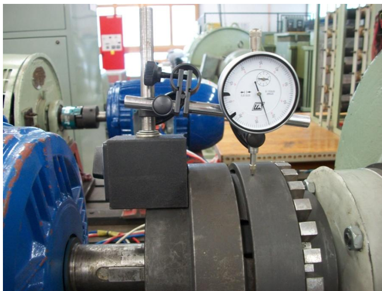
Figure 7.2: Motor and dynamometer shafts with alignment clock
