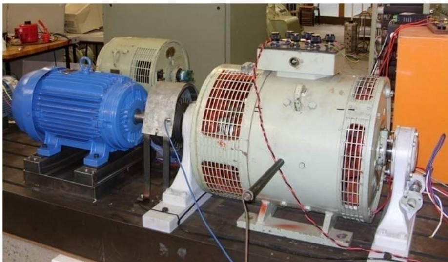
Figure 7.1: Test rig with dynamometer coupled to an induction motor
