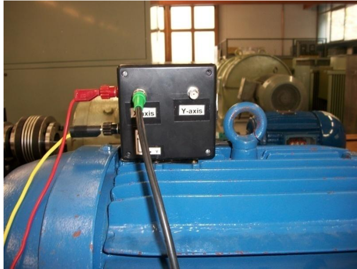
Figure 7.10: Accelerometer device placed on an induction machine
