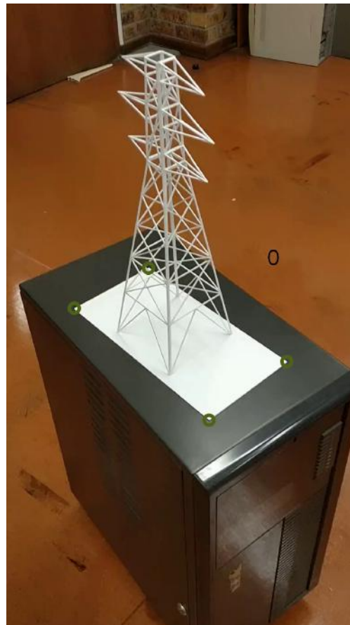
FIGURE 6.5: An image of a pylon mounted on a platform. The four corners of the platform marked as shown in the figure are used to derive the ground truth pose needed to test the algorithms .
