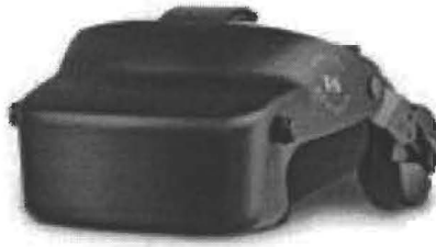
Figure 2: Head Mounted Display (HMD) . It is a V6 Head Mounted Display manufactured by Visual Research.
