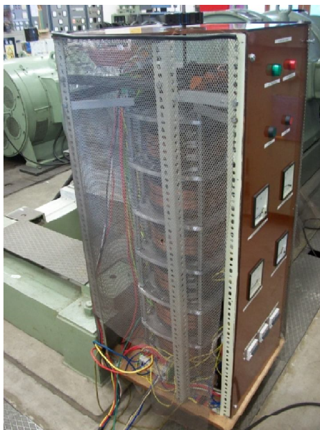
Figure 15: 40kVA three-phase series connected variac
