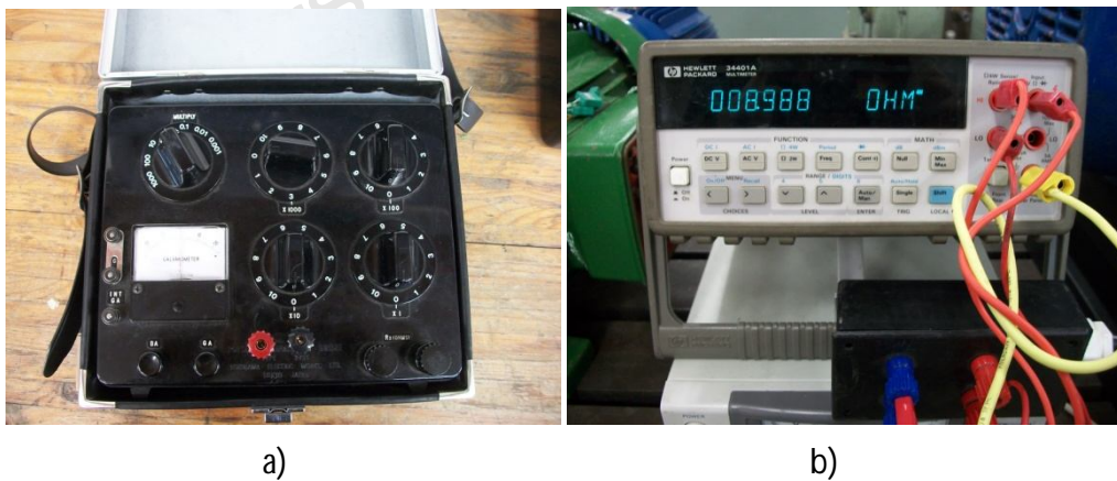
Figure 23: a) Galvanometer and b) Digital Multi Meter for winding resistance measurement
