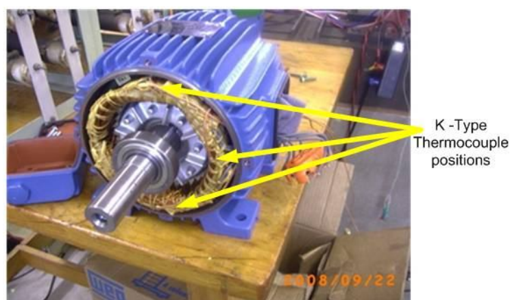
Figure 26: Thermocouple placement on stator end windings
