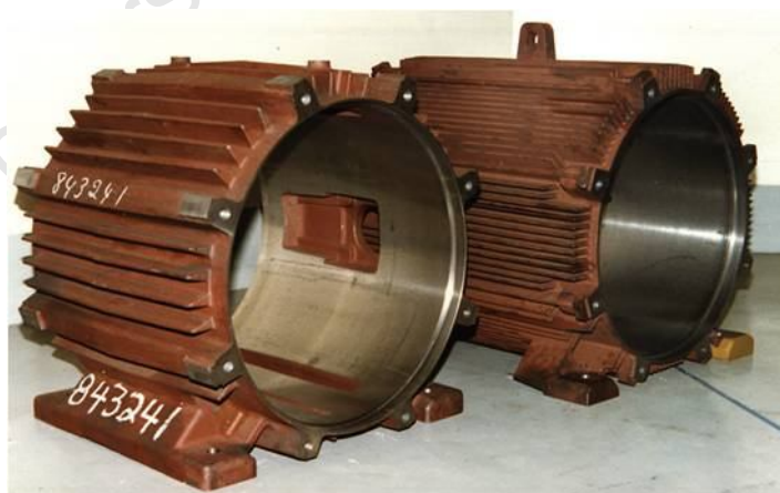
Figure 31: EE Motor casing with more ribs to improve surface area
