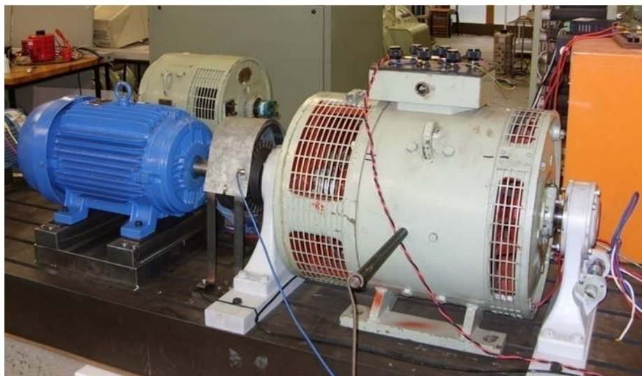
Figure 13: 15kW Test rig – Dynamometer coupled to a standard induction motor
