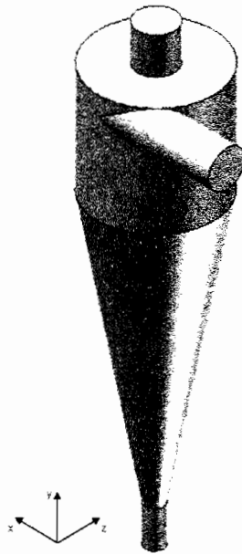
Figure 3.1: Basic CFD cyclone model geometry
