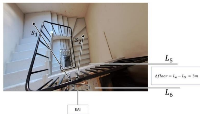
Figure 6-5: Experimental set-up for vertical distance using outside staircase.
