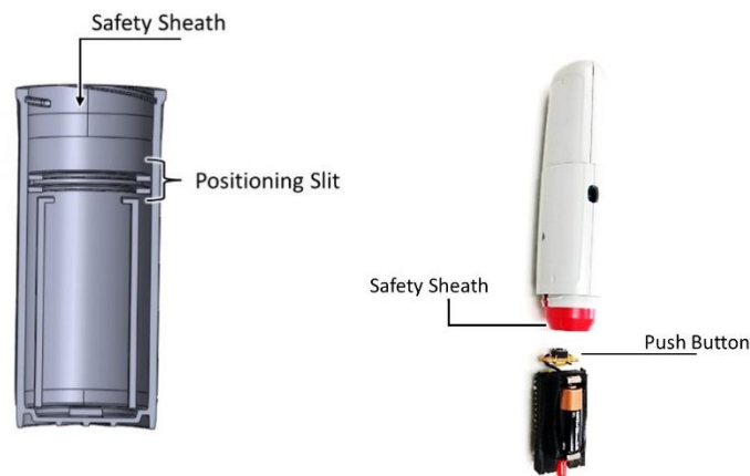
Figure 5-12: Slit design for fixed positioning of the tactile button.
