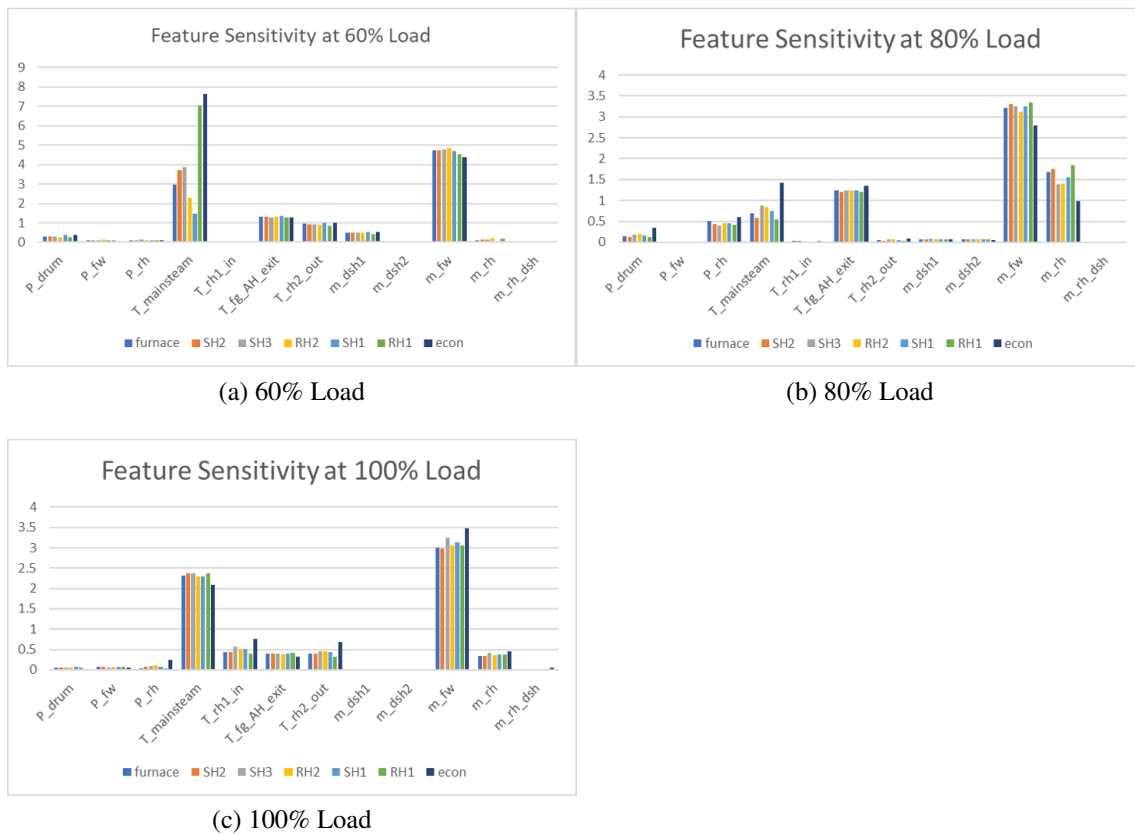
Figure 12: Sensitivity analysis without excess air ratio ( \alpha ) shown
