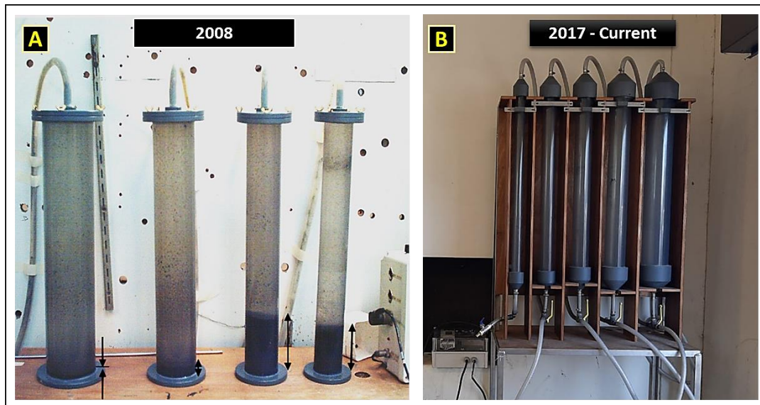
Figure 2.7: The UCT- settleometer: (A) earlier four-column design and (B) current five-column design.
