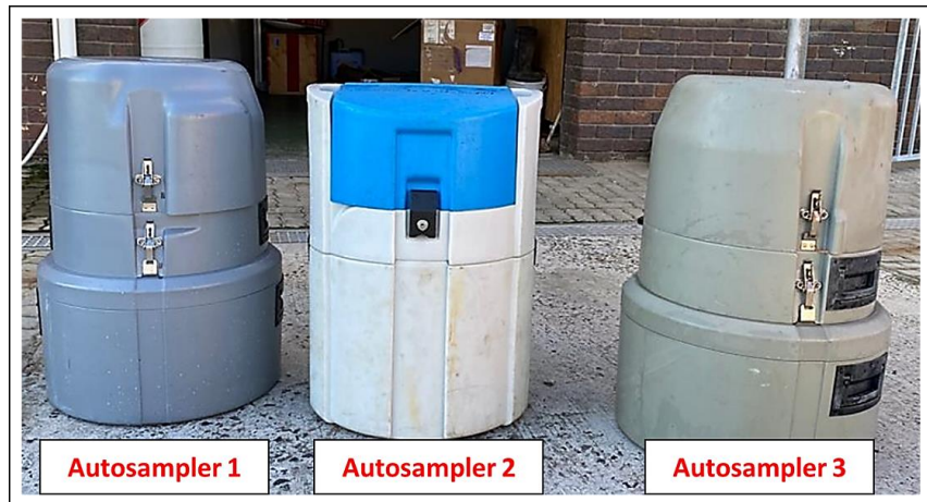
Figure 3.15: The three selected autosamplers for the influent, underflow, and effluent flow automatic sampling
