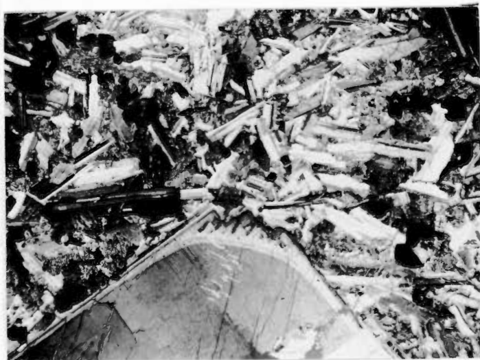
No. 27. The Gamsbokberg dolerite showing part of a plagioclase phenocryst. Crossed Nicols. x20.
