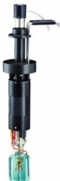
Figure 3-6: The 100 mL reaction vessel with the sample ampoule attached and ready to be inserted into the thermostat.
