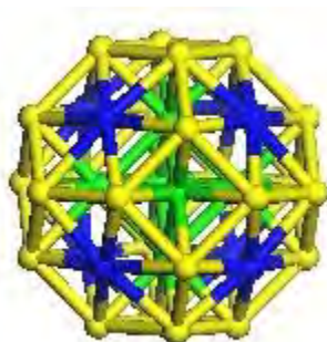
Figure 3.2: Different atomic orbits in a 38 atom truncated octahedron cluster, the three different orbits are represented by the green (coordination number 12), blue (coordination number 9) and yellow atoms (coordination number 6).
