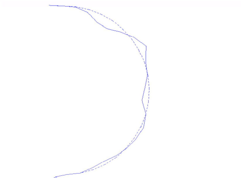
Figure 6.6: Kouga dam mode shape at 8.57 Hz
