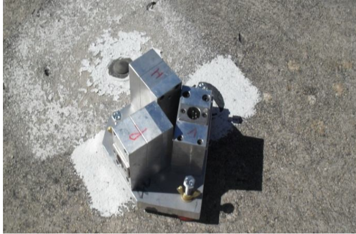
Figure 5.7: Forced balanced accelerometers
