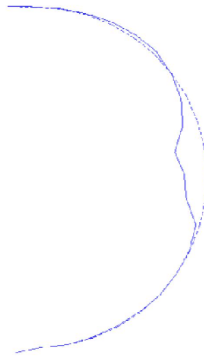
Figure 6.3: Kouga dam mode shape at 4.09 Hz
