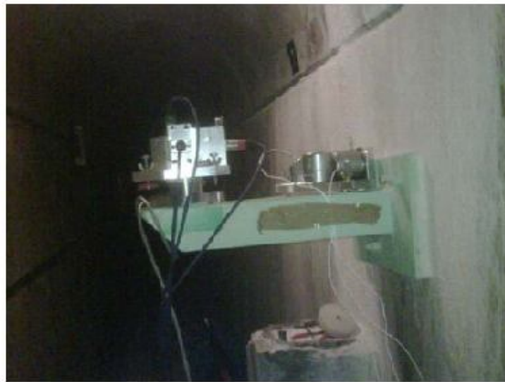
Figure 5.12: Arrangement of accelerometers mounted on a geodetic survey bracket
