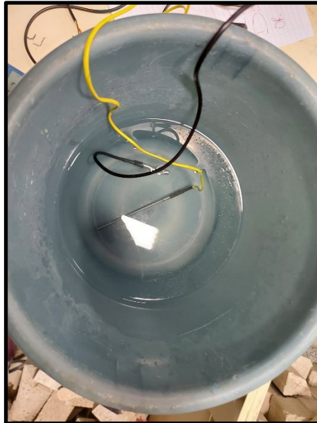
Figure K-2: Setup for Accuracy and Precision Testing for DS18B20
