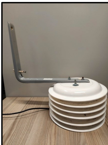
Figure 4-22: Radiation Shield Built to House Temperature and Humidity Sensor
