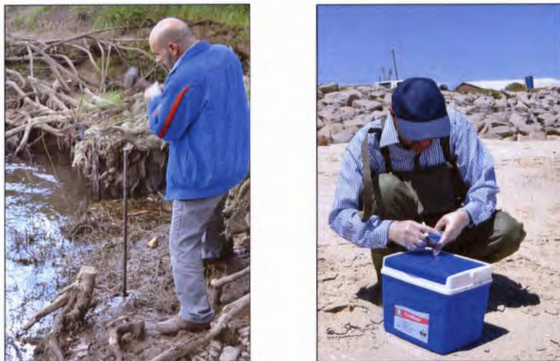
Figure 2.3.2 Inserting the short corer on the left and Storage of sub- samples on the right
