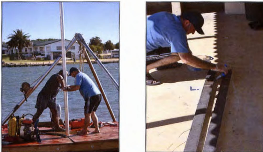
Figure 2.3.3 Vibracores collection on the left and selected subsamples on the right.
