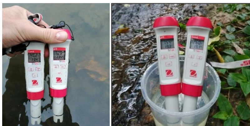
Figure 4-6: OHAUS® hand-held probes for Temperature, EC, and pH
