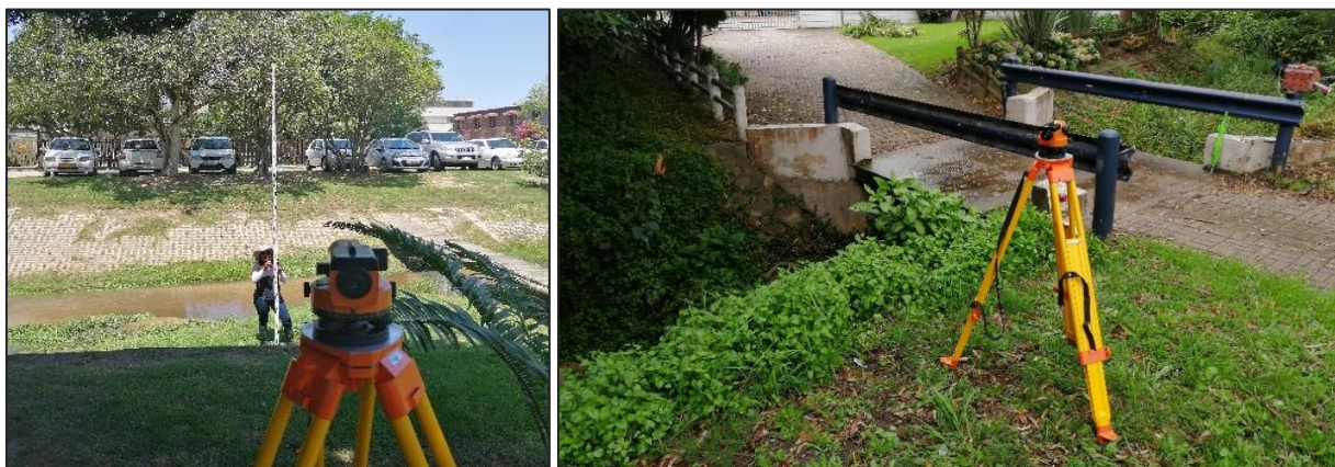
Figure 4-5: Dumpy level, tripod, and incremented survey staff
