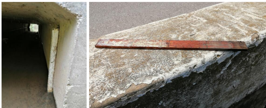
Figure 4-4: Chalk stick measurement device beneath George Rex Drive
