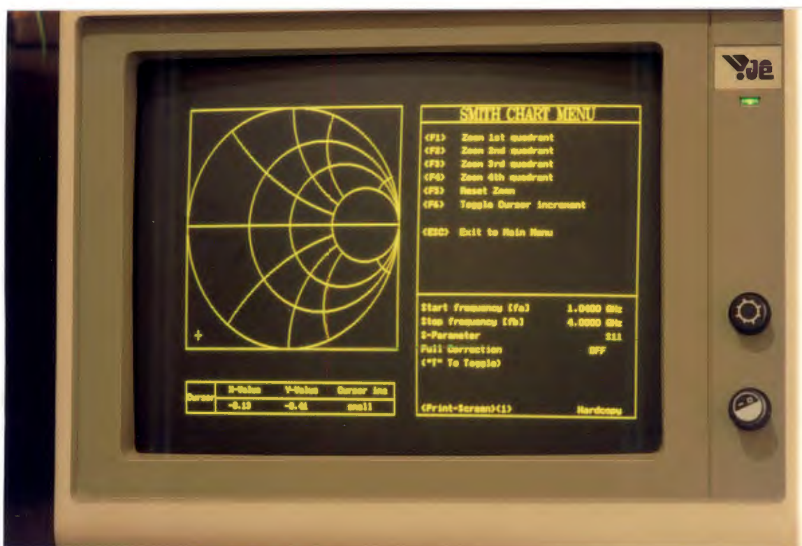
Figure 4.17. Real-Time Smith Chart Display.
