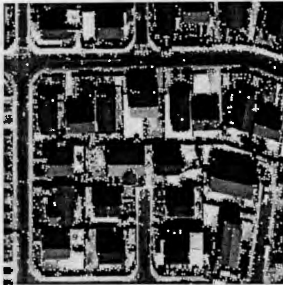
Figure 6.8: An aerial image of an urban environment with Förstner interest points overlaid, to illustrate the effect of the detection of non interest points and the non detection of obvious interest points.
