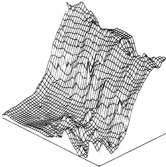
Figure 8.9: An orthographic plot of the Tygerberg Hills quarry test surface generated by the Surfer surface display package.
