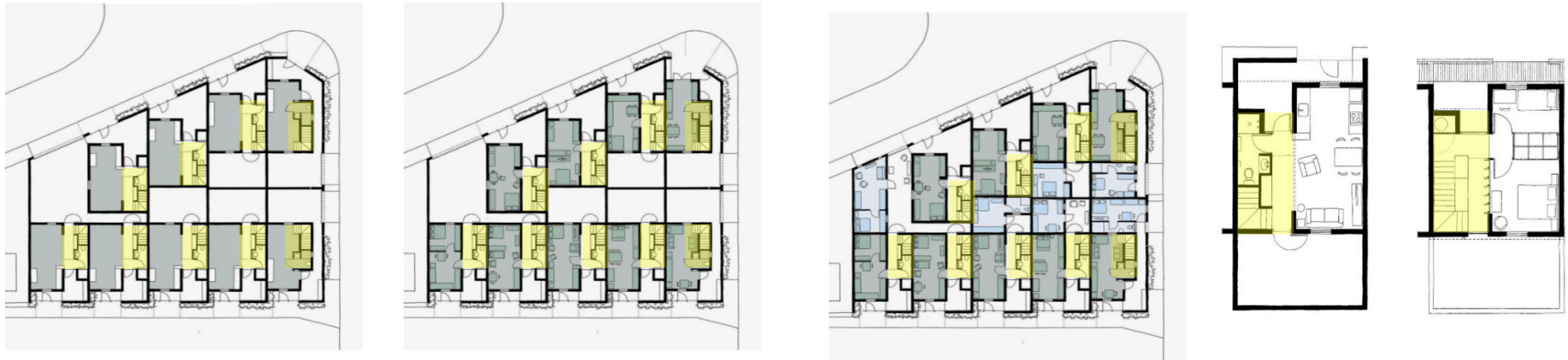
FIGURE 91: Floor Plans of Fenwick Lane, Highlighting the Separation of Service Spaces into Volumes Separate from The Rest of The Living Spaces
