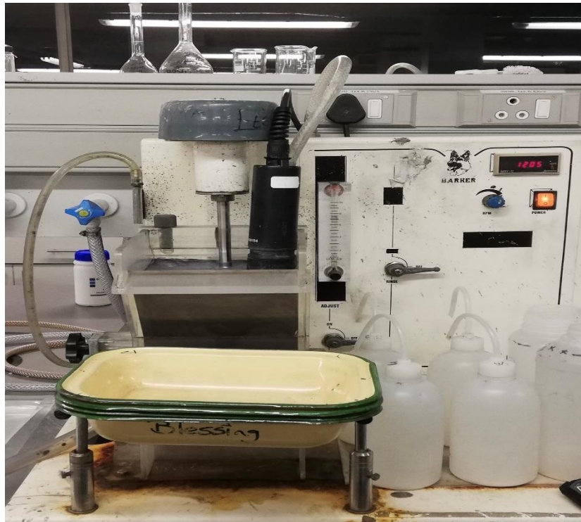
Figure 4- 3: The UCT 3L Barker laboratory flotation cell.
