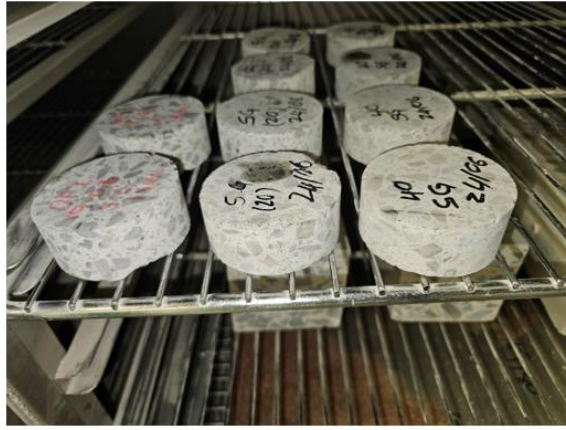
Concrete cores in oven during sample preparation
