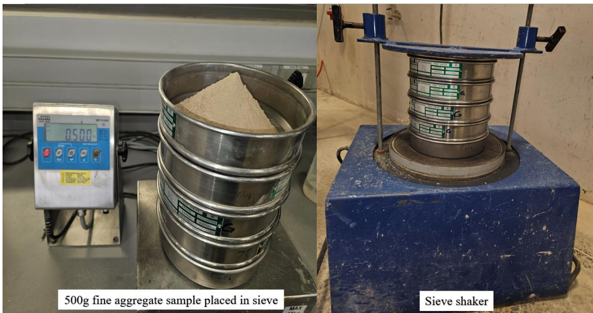
Figure 3-4: Apparatus used in particle size distribution test
