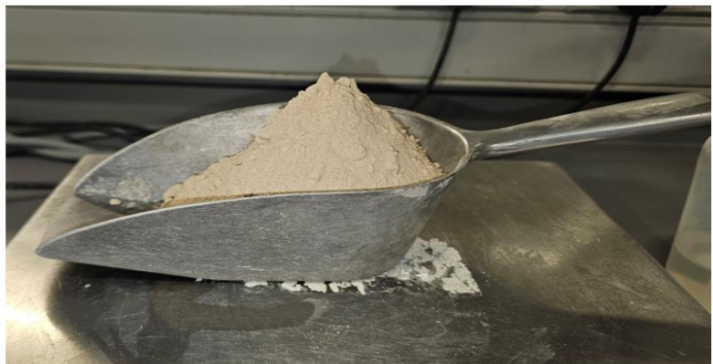
Gold mine tailings being weighed for use in this experiment
