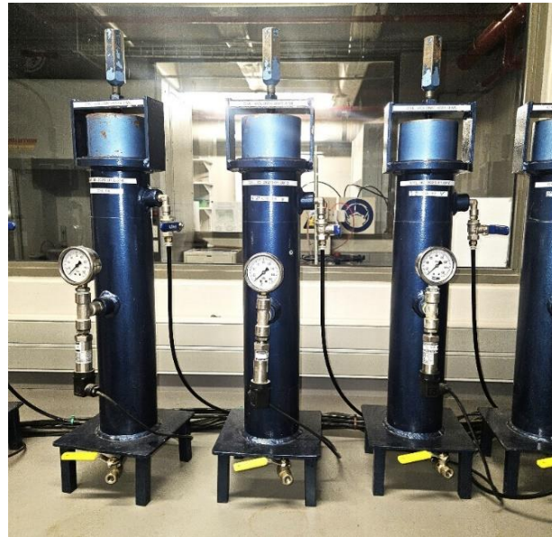
Figure 3-12: OPI testing apparatus
