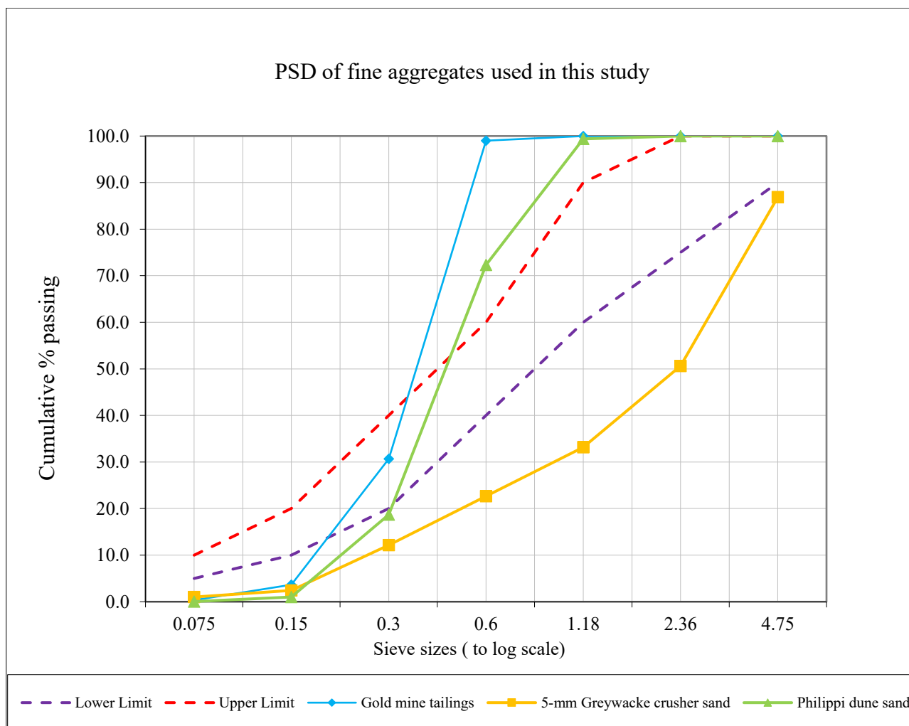
Figure 4-1: PSD graphs of fine aggregates used in this study
