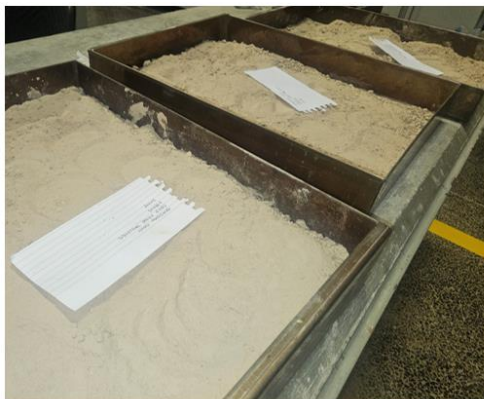
Gold mine tailings after oven drying used in this experiment
