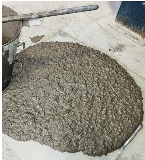
Figure 4-3: Visual representation of the sticky and non-cohesive concrete observed at higher replacement ratios
