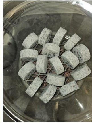
Concrete cores in desiccator during sample preparation
