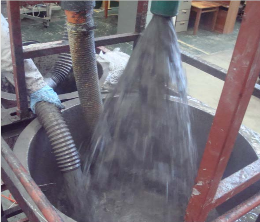
Figure 4-20. Main sump with U/F and O/F streams
