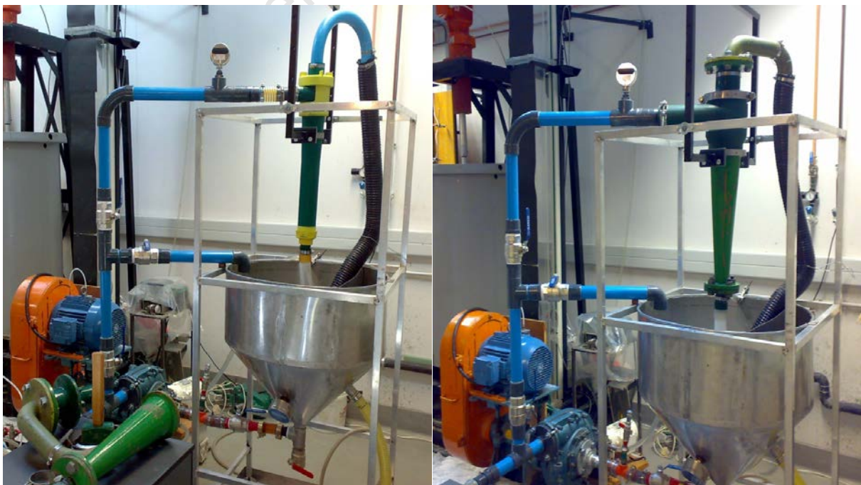
Figure 4-17. UCT cyclone rig with 75 mm cyclone (left) and 100 mm cyclone (right).
