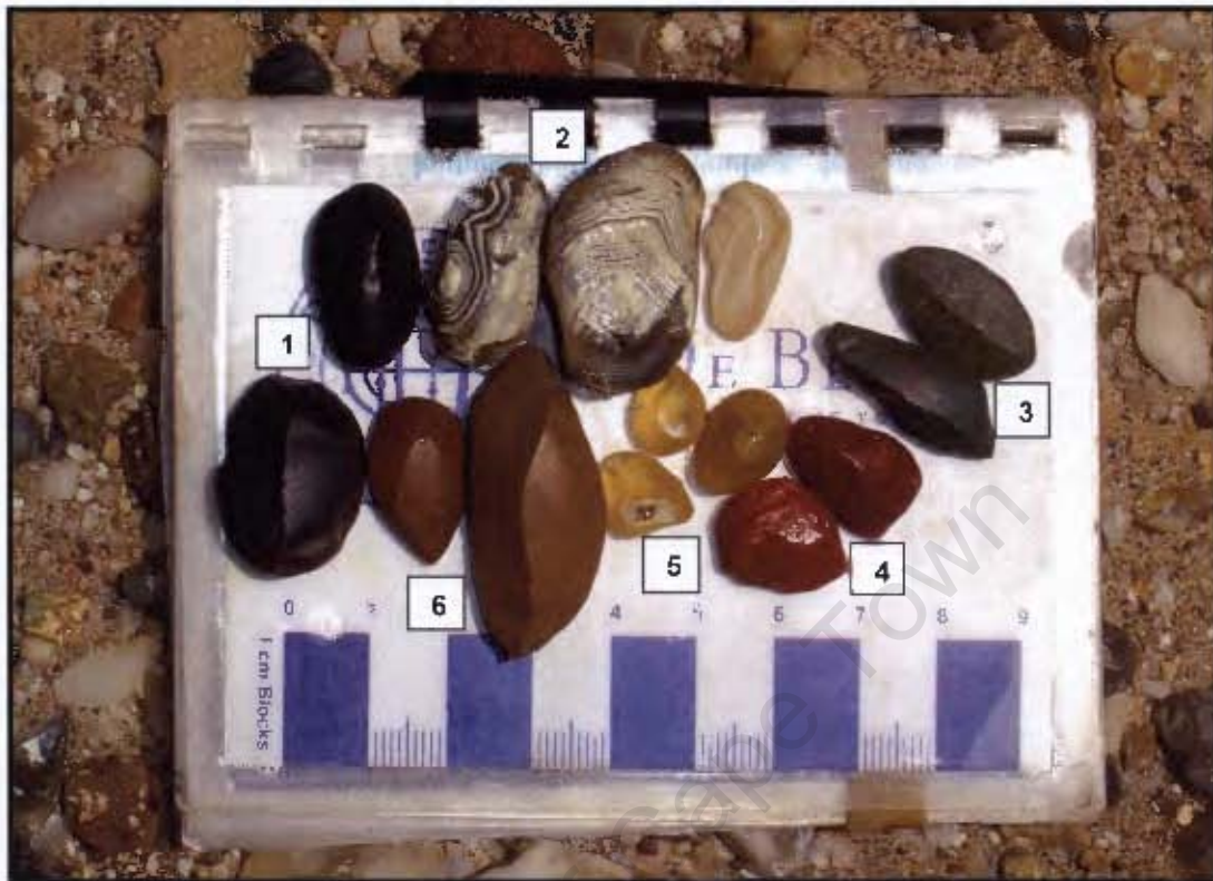
Figure 4.20: Ventifacted exotics from the remnant Eocene shoreline at Lüderitzkrater bearing evidence of the aggressive wind regime in the central Sperrgebiet. Exotics photographed include, 1. black chert; 2. agate; 3. chrysoprase; 4. jasper; 5. yellow chalcedony and 6. lutite banded ironstone formation
