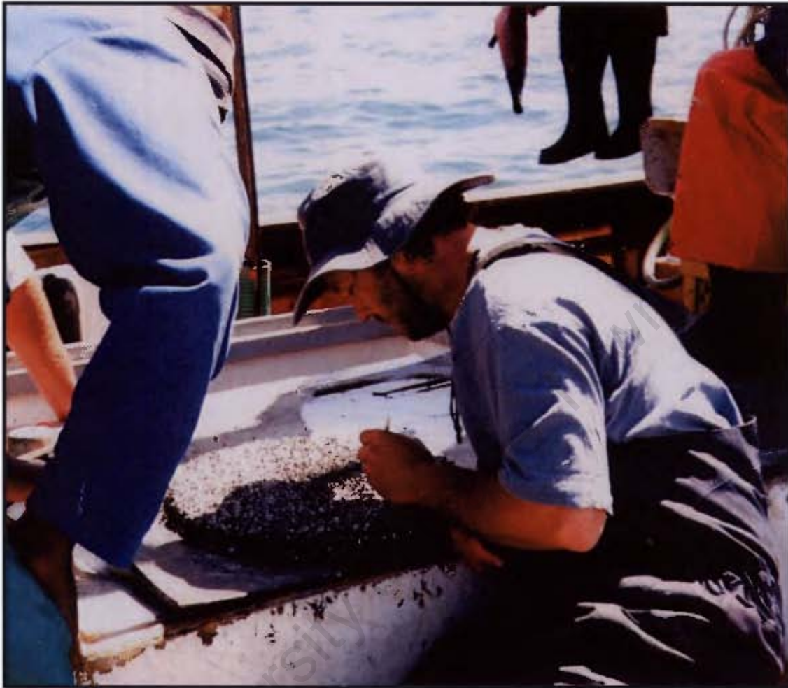
Figure 6.2: A diver (B. Mitchell) sorting through jiggled concentrate for diamonds onboard the mv Rachel while mining of De Hoek. See Figure 4.1.
