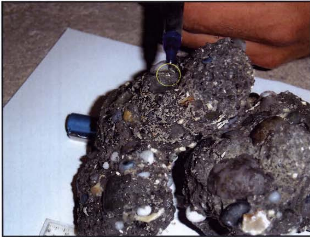
Figure 7.15: Hand specimen of cemented gravel recovered from -26 m depth in a gully at De Hoek – small diamond in the matrix indicated by the pen.
