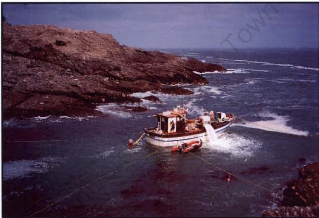
Figure 7.17: Facing south-west, the mv Rachel mining shallow deposits in the narrow confines of De Hoek 1 on a very calm day (see Figure 7.11). The divers had to place several mooring lines on land to secure the vessel in position.
