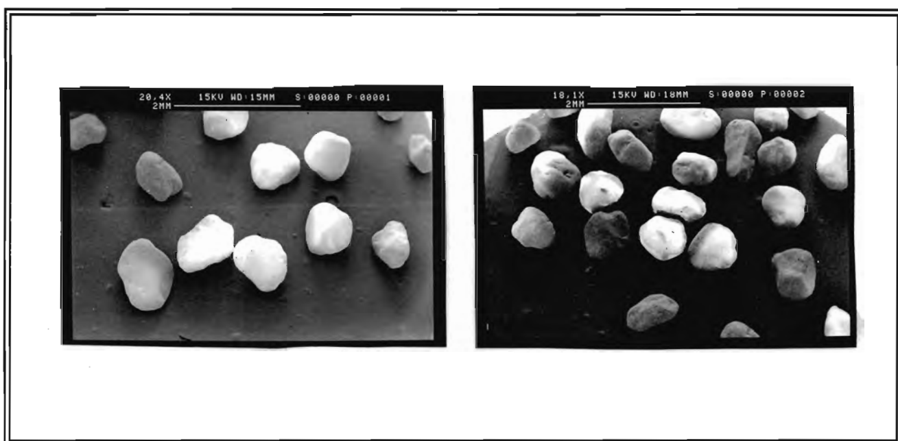
Figure 4.7. Electron micrographs of the silica particles used in this study.
